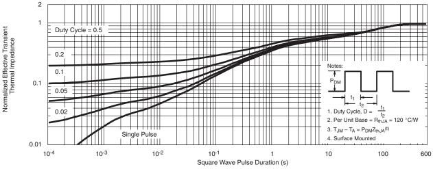
Normalized Thermal Transient Impedance, Junction-to-Ambient
