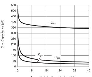
V<sub>DS</sub> - Drain-to-Source Voltage (V) **Capacitance**
