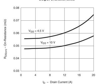
On-Resistance vs. Drain Current and Gate Voltage
