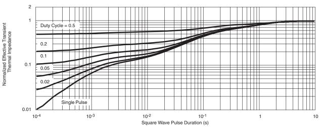
Normalized Thermal Transient Impedance, Junction-to-Case
