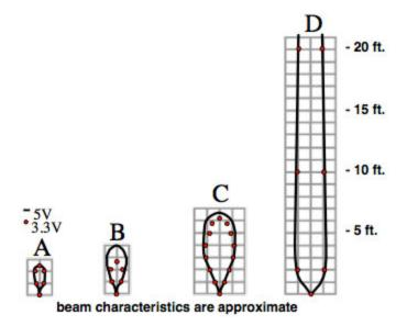
The different LV models have different beam width patterns, check this image for a comparison of all the LV model beam patterns. For higher sensitivity, check out the HR-LV models - they have up to 1mm sensitivity and 5 meter range!
