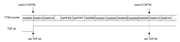
Figure 37-170. Example of up counting when the value of CNTIN is greater than the value of MOD
