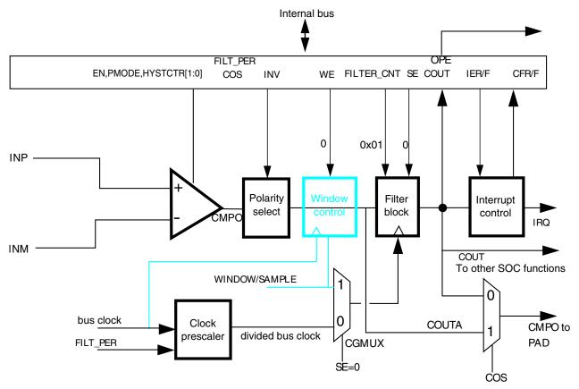
Figure 33-29. Sampled, Non-Filtered (# 3B): sampling interval internally derived
