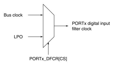
Figure 5-4. PORTx digital input filter clock generation
