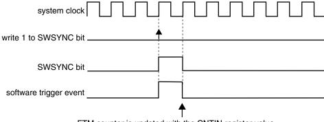
FTM counter is updated with the CNTIN register value and channel outputs are forced to their initial value
