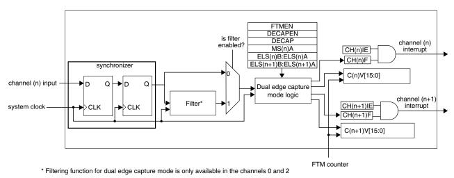
Figure 37-244. Dual Edge Capture mode block diagram
