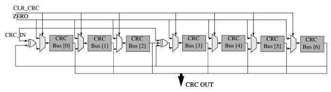
Figure 49-34. Command CRC Shift Register
