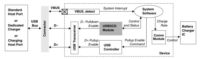
Figure 43-8. USB battery charging subsystem
