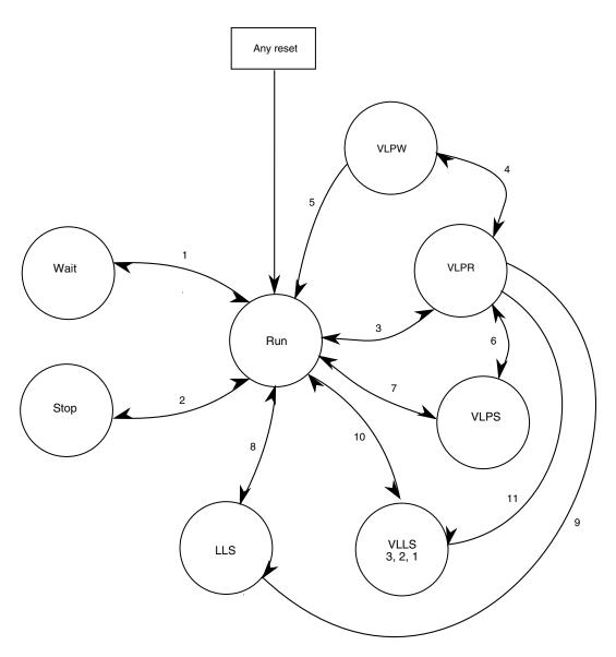
Figure 7-1. Power mode state transition diagram
