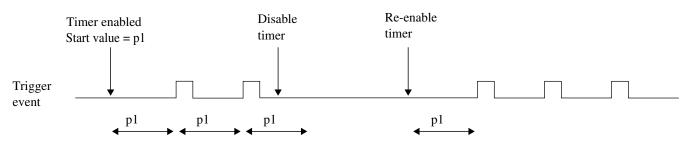
Figure 38-23. Stopping and starting a timer
