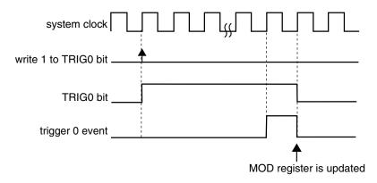
Figure 37-212. MOD synchronization with (SYNCMODE = 0), (HWTRIGMODE = 0), (PWMSYNC = 0), (REINIT = 1), and a hardware trigger was used
