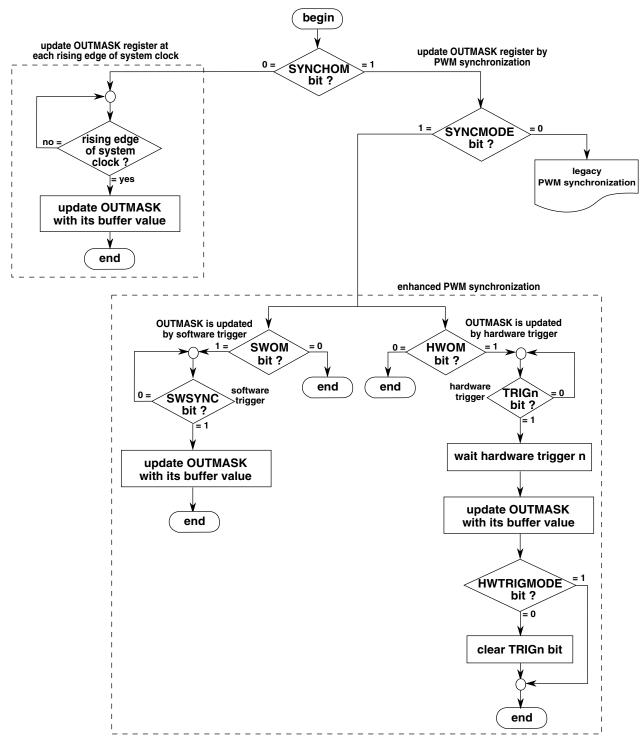
Figure 37-214. OUTMASK register synchronization flowchart
