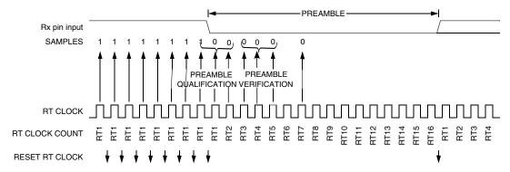
Figure 48-340. Receiver data sampling
