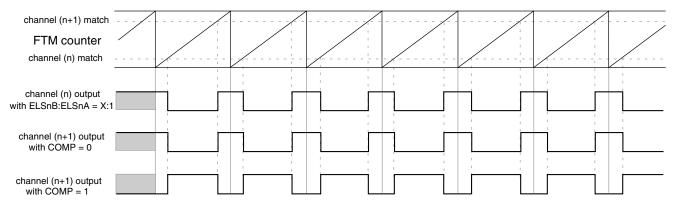
Figure 37-204. Channel (n+1) output in Complementary mode with (ELSnB:ELSnA = X:1)
