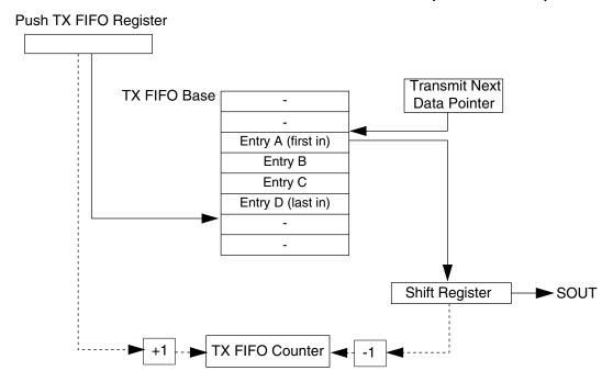
Figure 46-99. TX FIFO pointers and counter
