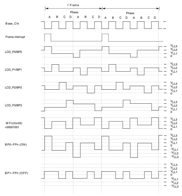
Figure 53-30. 1/4 duty and 1/3 bias (low-power waveform)
