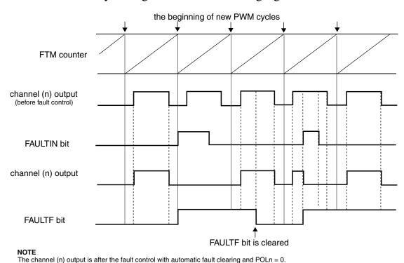
Figure 37-235. Fault control with automatic fault clearing
