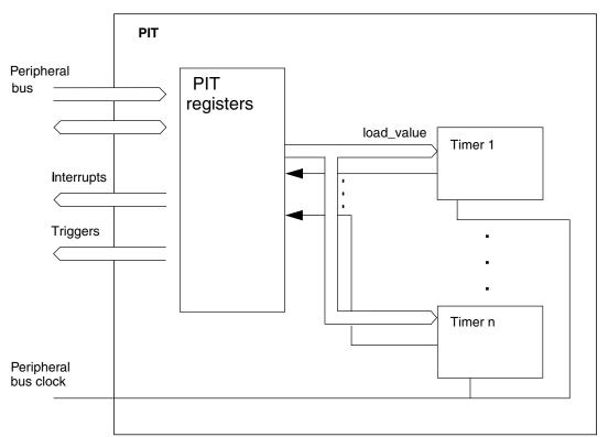
Figure 38-1. Block diagram of the PIT
