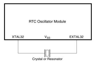
Figure 27-2. Crystal Connections
