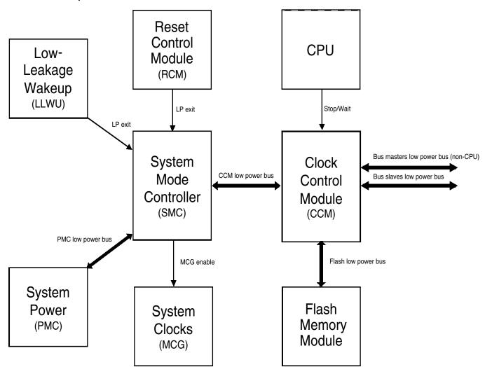
Figure 14-6. Low-power system components and connections
