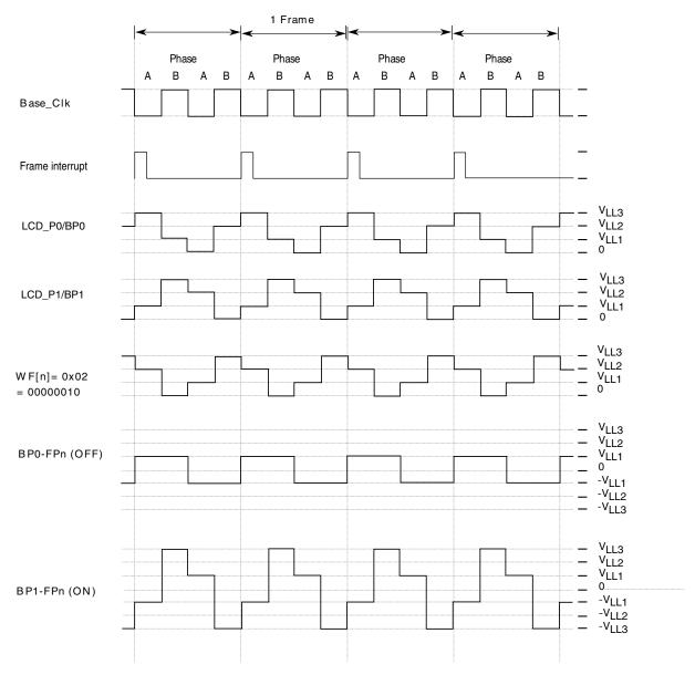
Figure 53-29. 1/2 duty and 1/3 bias (low-power waveform)
