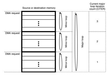
Figure 22-292. Example of multiple loop iterations
