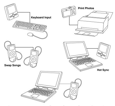
Figure 42-2. Example USB 2.0 On-The-Go configurations
