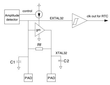
Figure 27-1. RTC Oscillator Block Diagram
