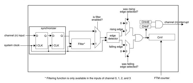
Figure 37-175. Input Capture mode
