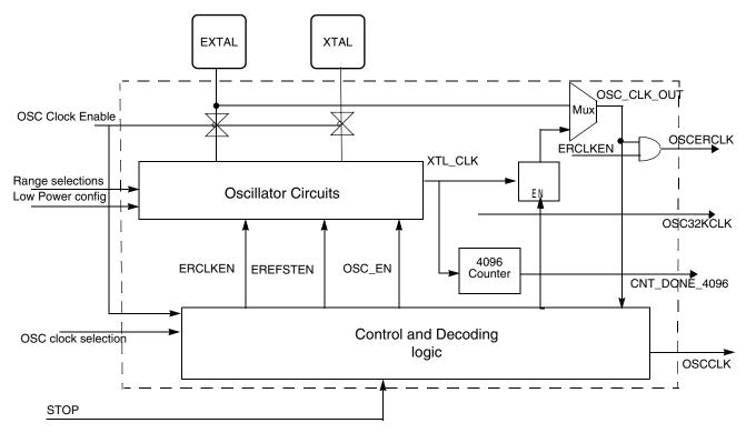
Figure 26-1. OSC Module Block Diagram
