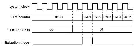
Figure 37-242. Initialization trigger is generated if (CNT = CNTIN), (CLKS[1:0] = 0:0), and a value different from zero is written to CLKS[1:0] bits
