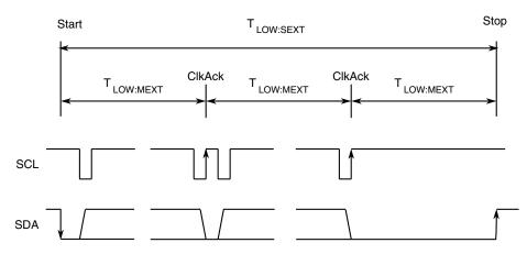
Figure 47-40. Timeout measurement intervals
