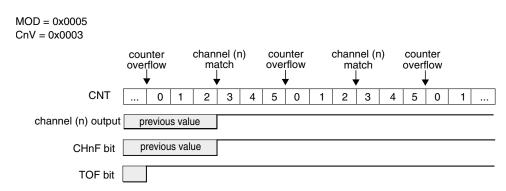
Figure 37-180. Example of the Output Compare mode when the match sets the channel output
