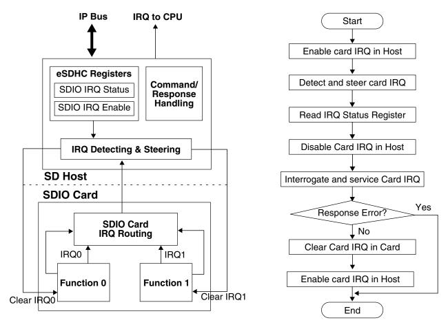
Figure 49-36. Card interrupt scheme and card interrupt detection and handling procedure
