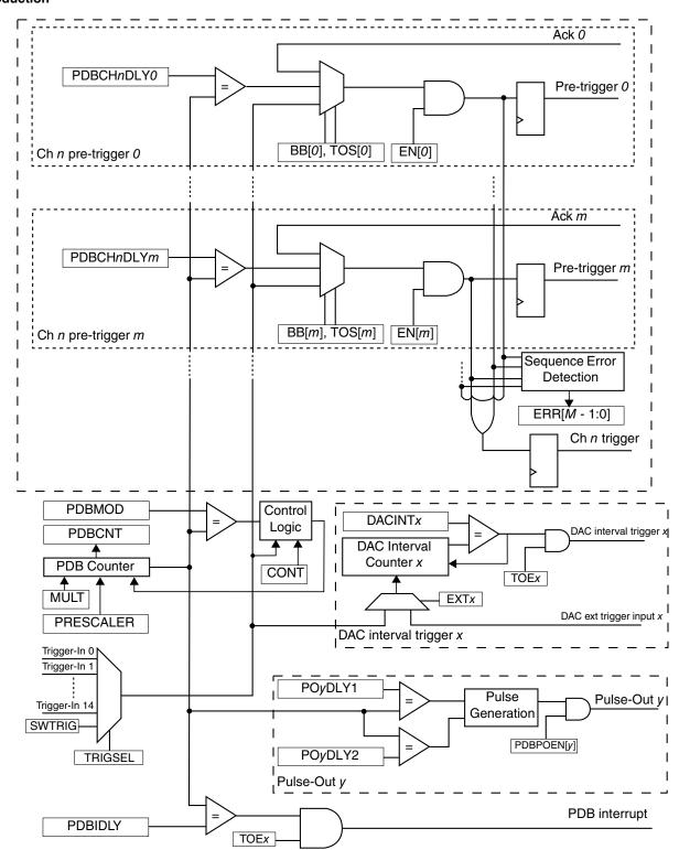
Figure 36-1. PDB block diagram
