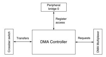
Figure 3-14. DMA Controller configuration
