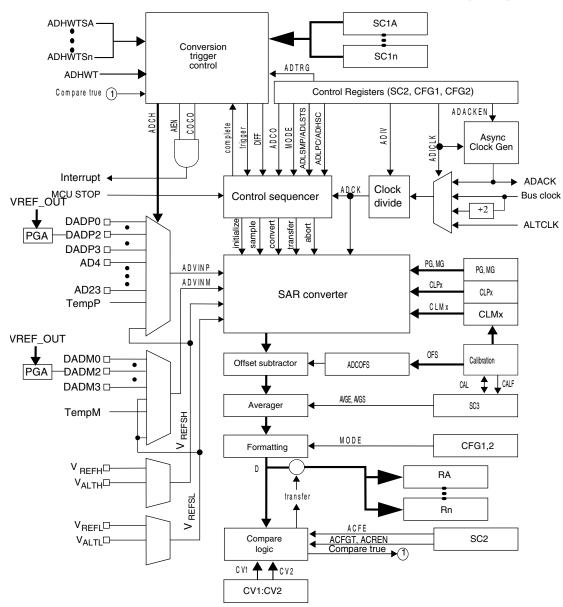
Figure 32-1. ADC block diagram
