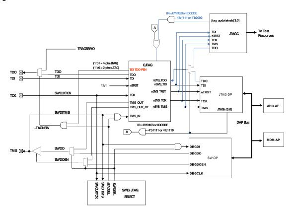
Figure 9-2. Modified Debug Port
