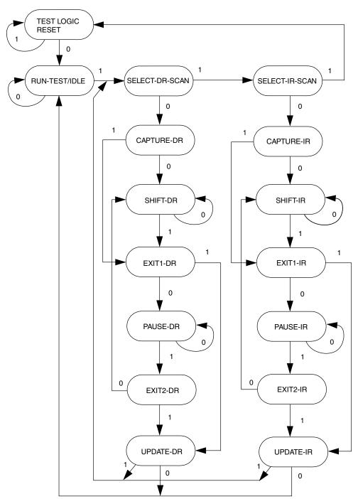
The value shown adjacent to each state transition in this figure represents the value of TMS at the time of a rising edge of TCK.
