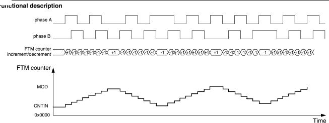
Figure 37-252. Quadrature Decoder – Phase A and Phase B Encoding mode
