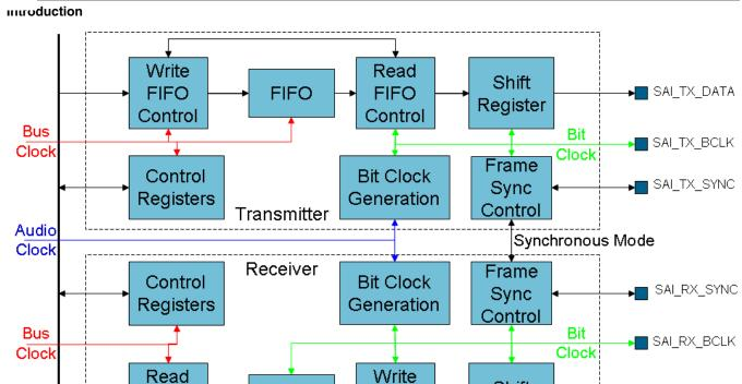
Figure 50-1. I<sup>2</sup>S/SAI block diagram
