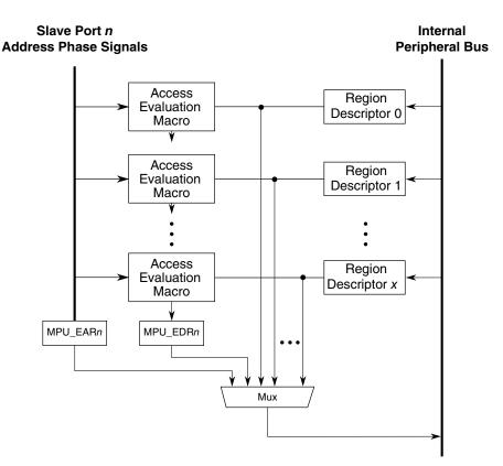
Figure 19-1. MPU block diagram
