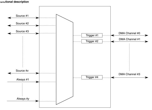
Figure 21-19. DMA MUX triggered channels
