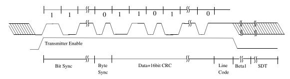
Figure 48-337. Frame format with differential manchester encoding
