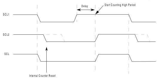
Figure 47-39. I2C clock synchronization
