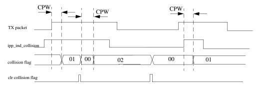
Figure 48-341. Collision pulse detection
