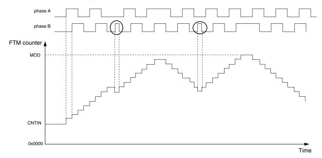
Figure 37-255. Motor position jittering in a mid count value
