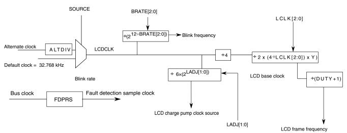
Figure 53-28. LCD clock tree
