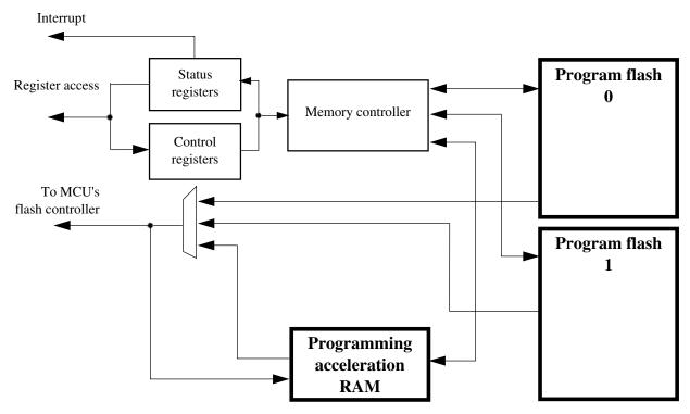
Figure 29-1. Flash Block Diagram
