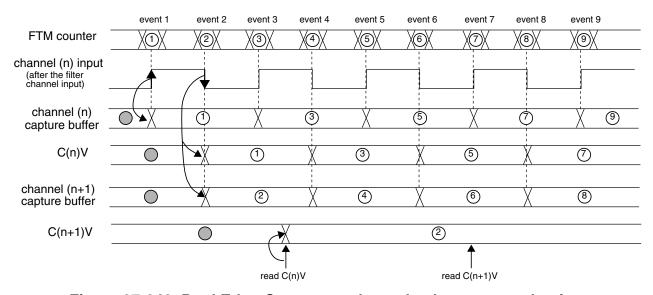
Figure 37-249. Dual Edge Capture mode read coherency mechanism
