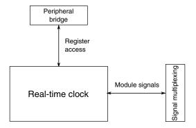
Figure 3-45. RTC configuration
