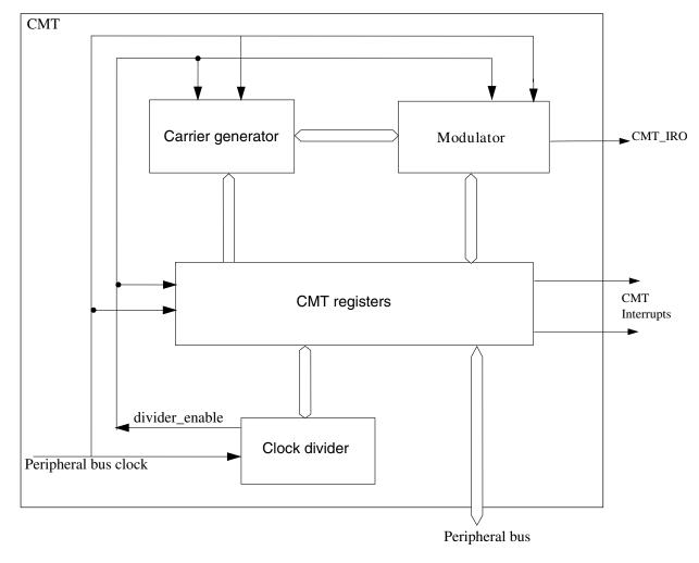
Figure 40-1. CMT module block diagram
