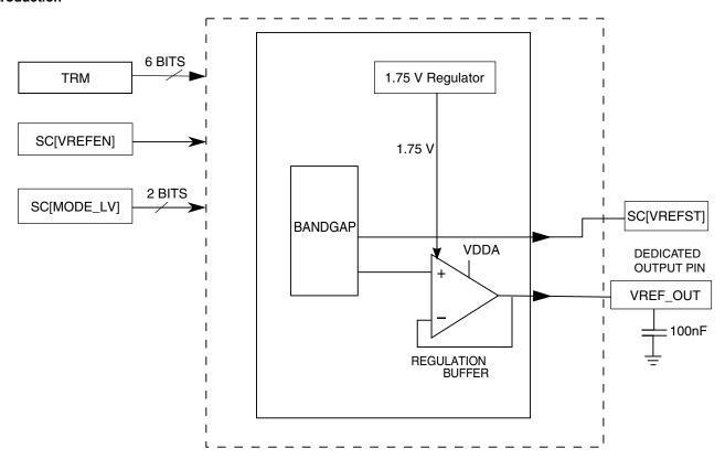
Figure 35-1. Voltage reference block diagram
