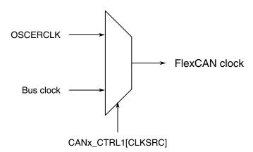
Figure 5-7. FlexCAN clock generation
