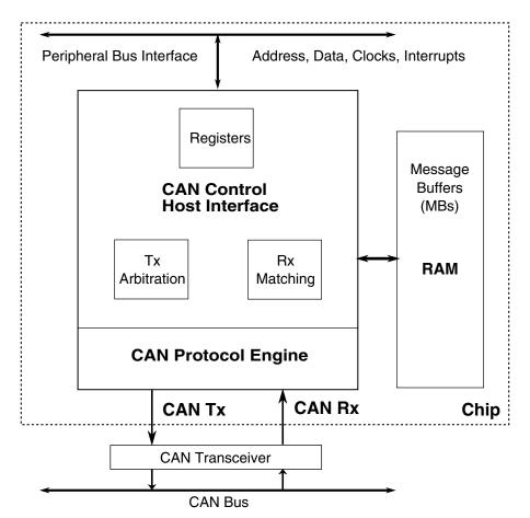
Figure 45-1. FlexCAN block diagram
