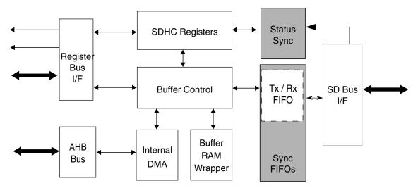
Figure 49-27. SDHC buffer scheme
