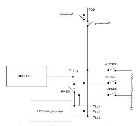
Figure 53-32. LCD charge pump block diagram
