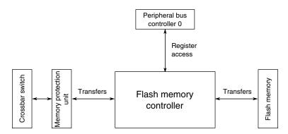
Figure 3-22. Flash memory controller configuration
