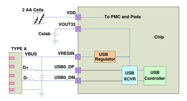
Figure 3-48. USB regulator AA cell usecase
