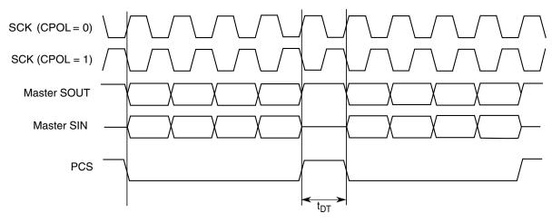
Figure 46-97. Continuous SCK Timing Diagram (CONT=0)
