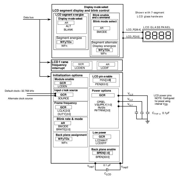
Figure 53-38. LCD programmer's model diagram
