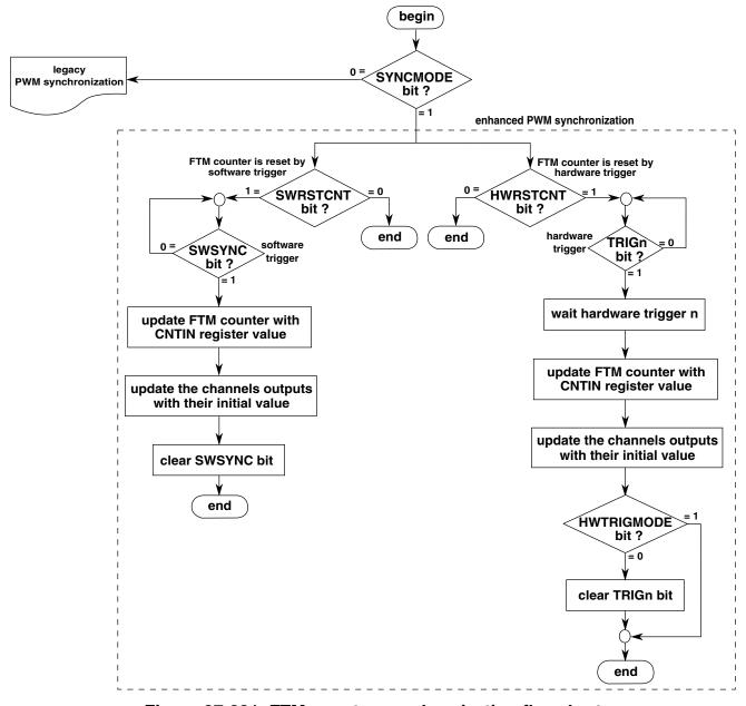
Figure 37-221. FTM counter synchronization flowchart
