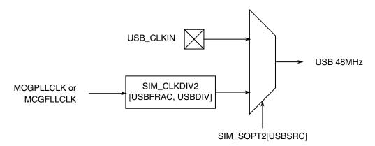
Figure 5-6. USB 48 MHz clock source
