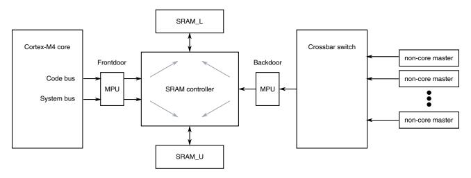
Figure 3-25. SRAM access diagram
