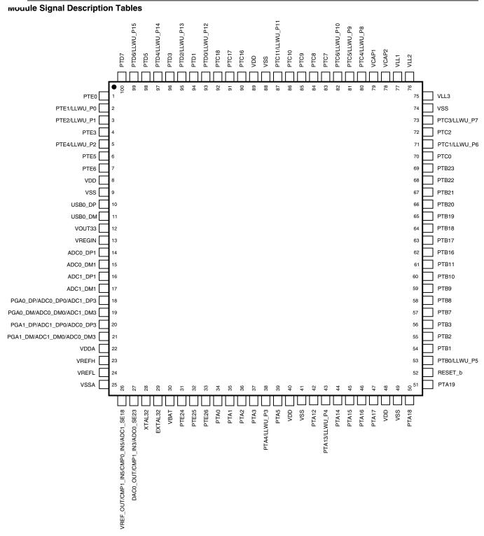
Figure 10-2. K40 100 LQFP Pinout Diagram
