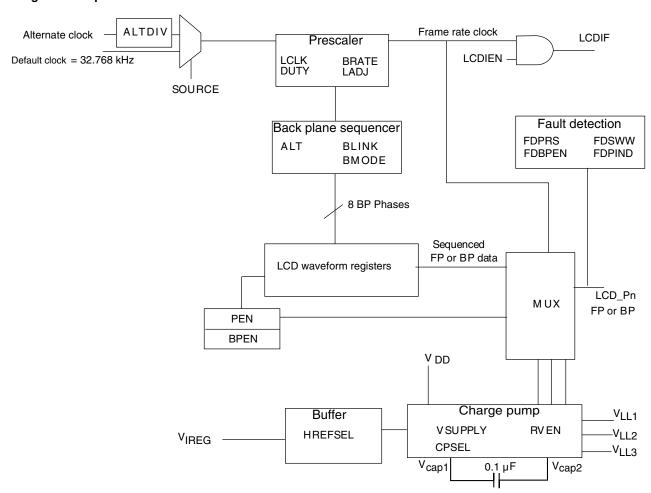
Figure 53-1. SLCD block diagram
