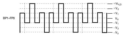
Figure 53-41. "f" segment voltage waveform
