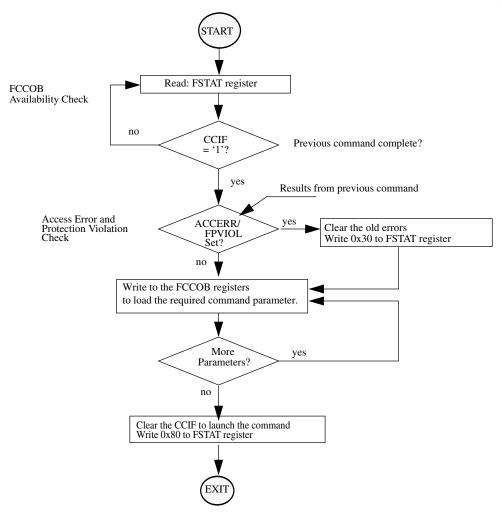
Figure 29-25. Generic Flash Command Write Sequence Flowchart
