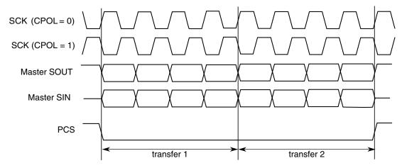
Figure 46-98. Continuous SCK timing diagram (CONT=1)
