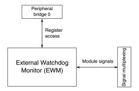
Figure 3-15. External Watchdog Monitor configuration
