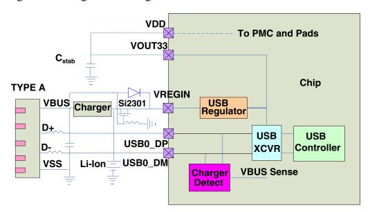
Figure 3-49. USB regulator Li-ion usecase
