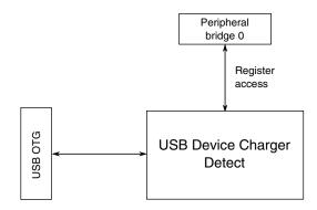
Figure 3-52. USB DCD configuration
