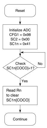
Figure 32-97. Initialization flowchart example
