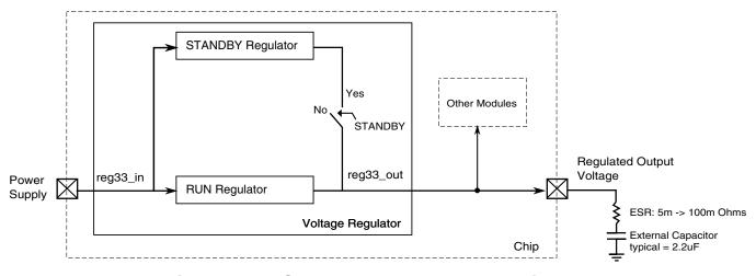
Figure 44-2. USB Voltage Regulator Block Diagram
