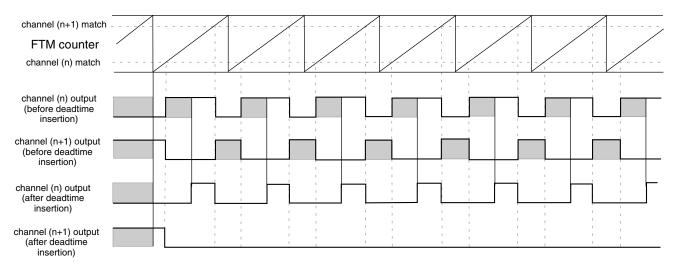
Figure 37-230. Example of the deadtime insertion (ELSnB:ELSnA = 1:0, POL(n) = 0, and POL(n+1) = 0) when the deadtime delay is comparable to channel (n+1) duty cycle
