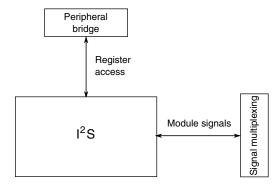
Figure 3-59. I<sup>2</sup>S configuration
