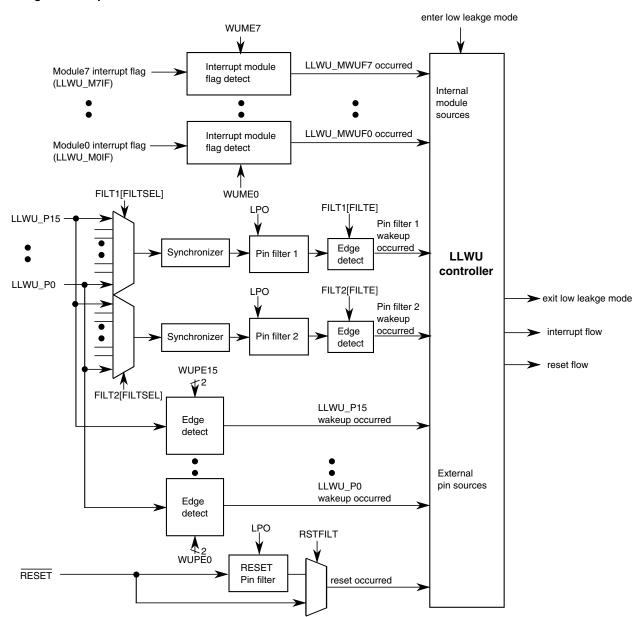
Figure 16-1. LLWU block diagram
