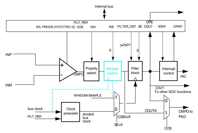
Figure 33-31. Sampled, Filtered (# 4B): sampling point internally derived
