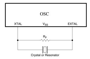
Figure 26-3. Crystal/Ceramic Resonator Connections - Connection 2
