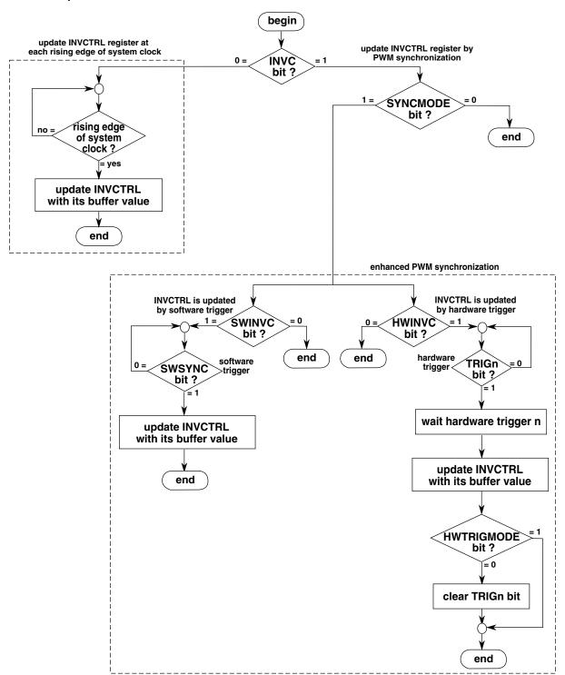
Figure 37-218. INVCTRL register synchronization flowchart
