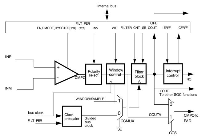
Figure 33-2. Comparator module block diagram
