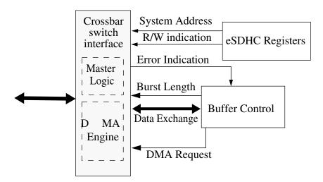
Figure 49-31. DMA crossbar switch interface block
