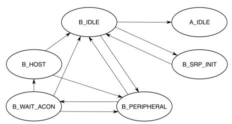
Figure 42-94. Dual role B device flow diagram
