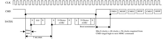
Figure 49-37. Multimediacard state diagram in Normal Boot mode
