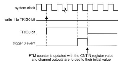
Figure 37-224. FTM counter synchronization with (SYNCMODE = 0), (HWTRIGMODE = 0), (REINIT = 1), (PWMSYNC = 1), and a hardware trigger was used
