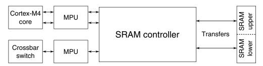
Figure 3-26. SRAM controller configuration
