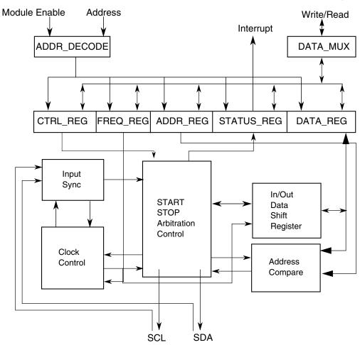
Figure 47-1. I2C Functional block diagram
