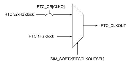
Figure 3-46. RTC\_CLKOUT generation
