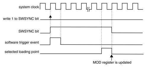
Figure 37-213. MOD synchronization with (SYNCMODE = 0) and (PWMSYNC = 1)
