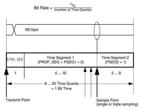
Figure 45-99. Segments within the bit time
