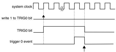
FTM counter is updated with the CNTIN register value and channel outputs are forced to their initial value
