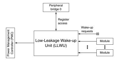
Figure 3-8. Low-Leakage Wake-up Unit configuration
