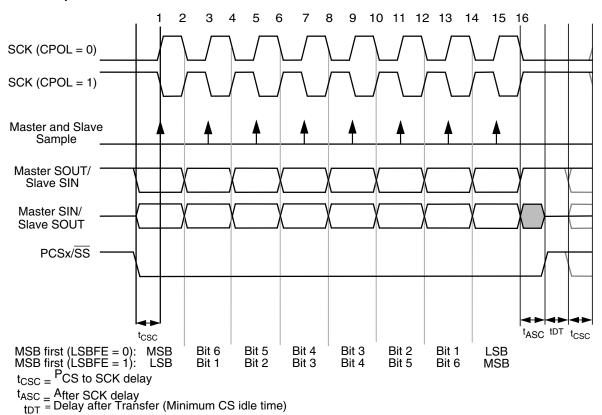
Figure 46-93. Module transfer timing diagram (MTFE=0, CPHA=0, FMSZ=8)
