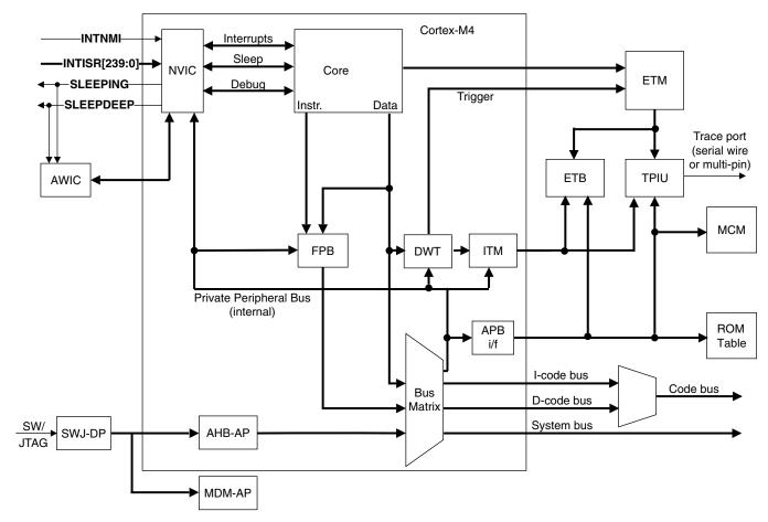
Figure 9-1. Cortex-M4 Debug Topology
