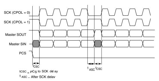
Figure 46-96. Example of continuous transfer (CPHA=1, CONT=1)
