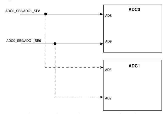
Figure 3-33. ADC hardware interleaved channels integration
