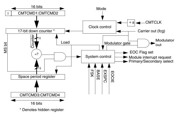
Figure 40-16. Modulator block diagram
