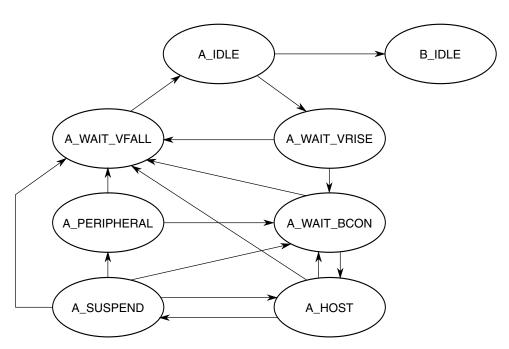
Figure 42-93. Dual role A device flow diagram
