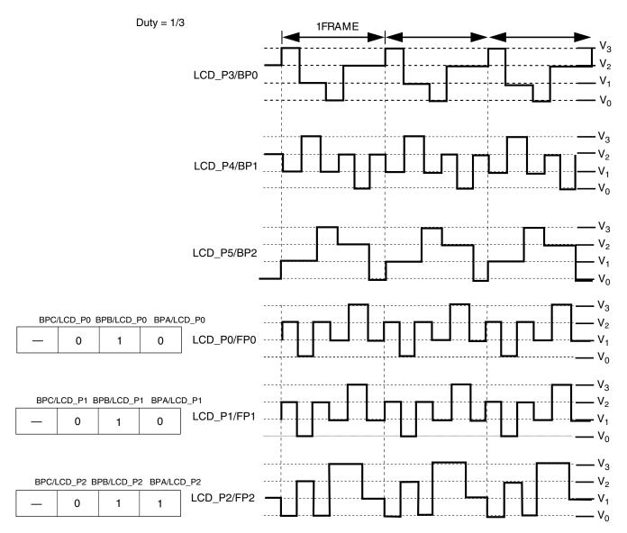
Figure 53-40. LCD waveforms
