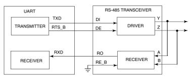
Figure 48-363. Transceiver driver enable using RTS
