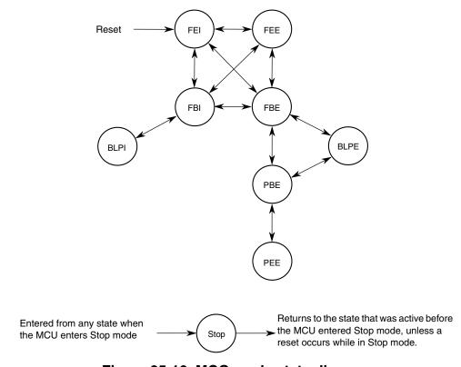
Figure 25-16. MCG mode state diagram
