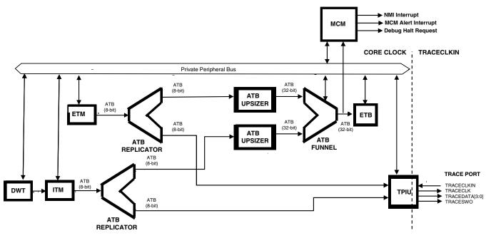
Figure 9-4. Core Trace Connectivity
