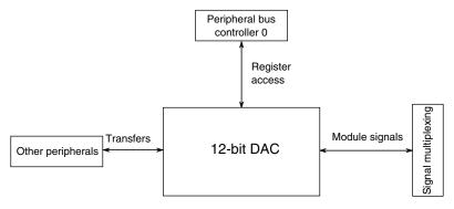
Figure 3-36. 12-bit DAC configuration
