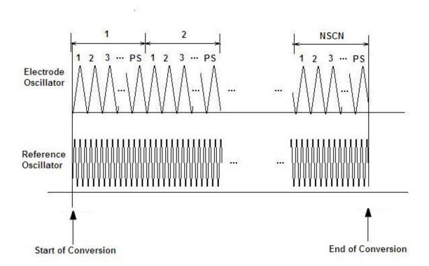
Figure 52-32. Dual electrode capacitance measurement
