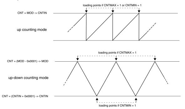
Figure 37-207. Boundary cycles and loading points
