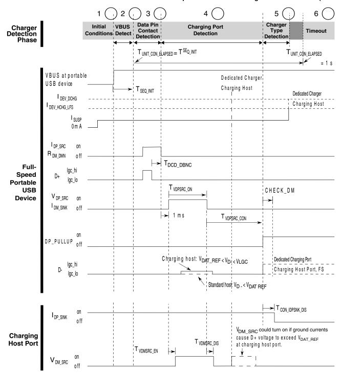
Figure 43-9. Full speed charger detection timing
