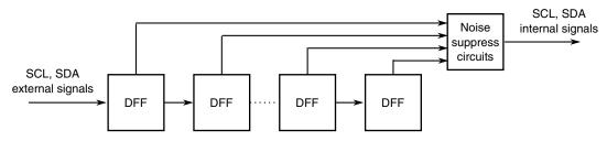
Figure 47-41. Programmable input glitch filter diagram
