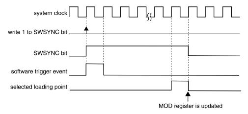
Figure 37-209. MOD synchronization with (SYNCMODE = 0), (PWMSYNC = 0), (REINIT = 0), and software trigger was used
