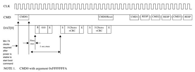
Figure 49-38. MultiMediaCard state diagram in Alternative Boot mode
