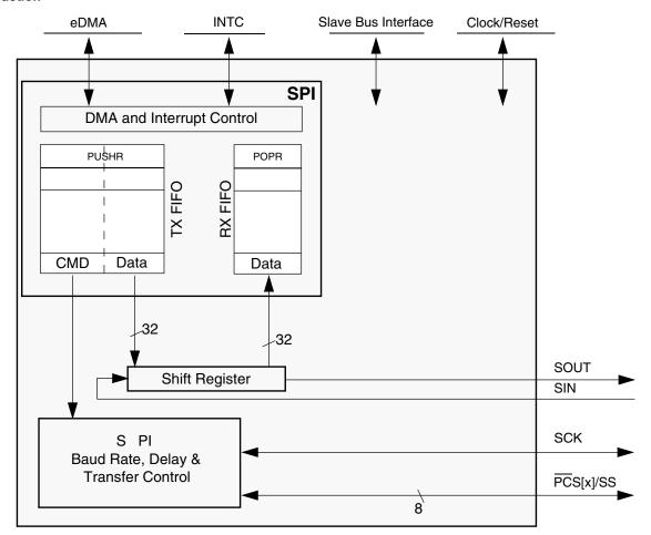
Figure 46-1. SPI Block Diagram
