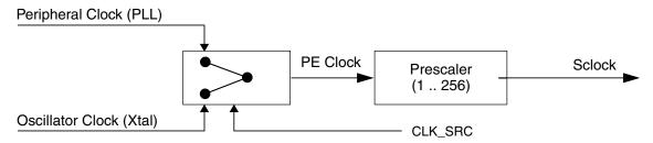
Figure 45-98. CAN engine clocking scheme
