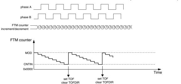
Figure 37-254. FTM counter overflow in down counting for Quadrature Decoder mode
