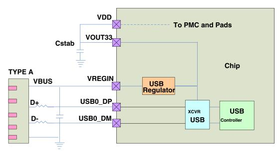
Figure 3-50. USB regulator bus supply
