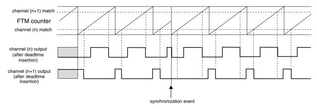
Figure 37-220. FTM counter synchronization
