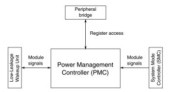
Figure 3-7. PMC configuration
