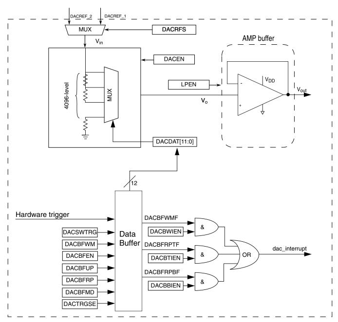
Figure 34-1. DAC block diagram
