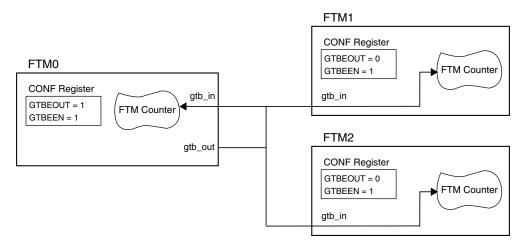
Figure 3-41. FTM Global Time Base Configuration
