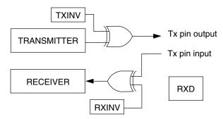
Figure 48-358. Single-wire operation (C1[LOOPS] = 1, C1[RSRC] = 1)
