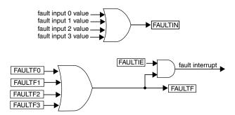
Figure 37-234. FAULTF and FAULTIN bits and fault interrupt
