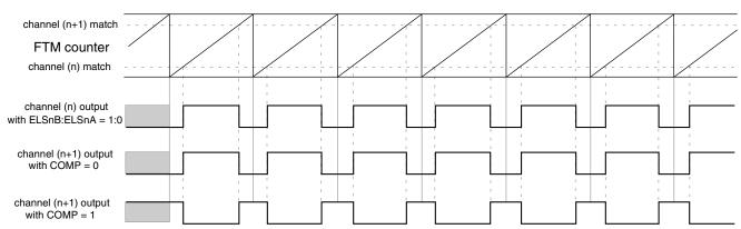
Figure 37-203. Channel (n+1) output in Complementary mode with (ELSnB:ELSnA = 1:0)
