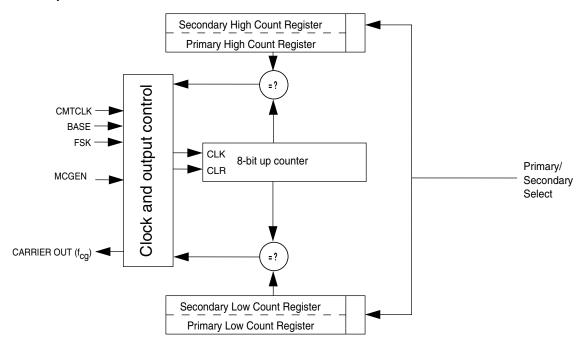
Figure 40-15. Carrier generator block diagram
