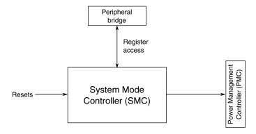
Figure 3-6. System Mode Controller configuration
