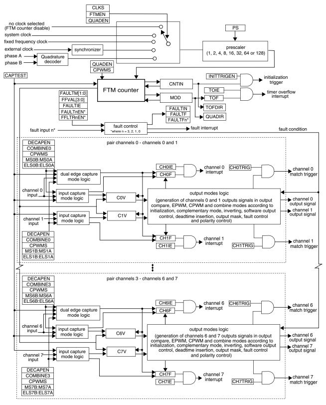
Figure 37-1. FTM block diagram
