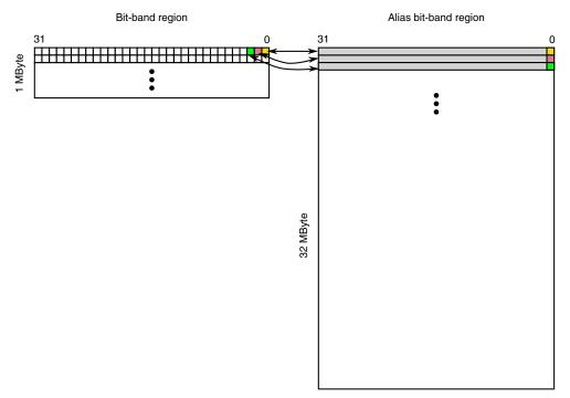
Figure 4-1. Alias bit-band mapping
