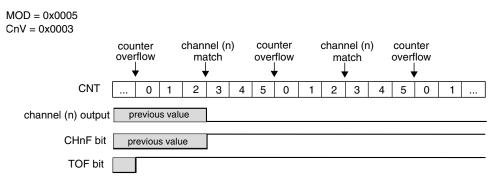
Figure 37-179. Example of the Output Compare mode when the match clears the channel output
