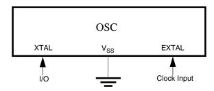
Figure 26-5. External Clock Connections
