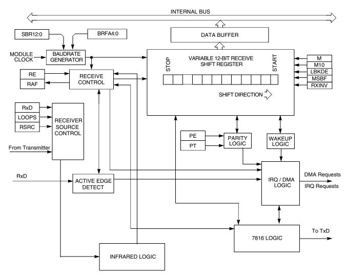
Figure 48-344. UART receiver block diagram
