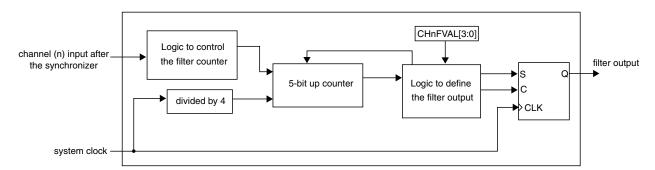
Figure 37-176. Channel input filter
