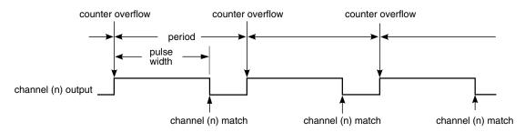
Figure 37-181. EPWM period and pulse width with ELSnB:ELSnA = 1:0
