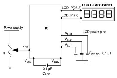
Figure 53-43. Power connections for contrast control
