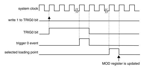
Figure 37-210. MOD synchronization with (SYNCMODE = 0), (HWTRIGMODE = 0), (PWMSYNC = 0), (REINIT = 0), and a hardware trigger was used
