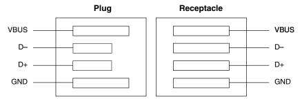
Figure 43-10. Relative pin positions in USB plugs and receptacles
