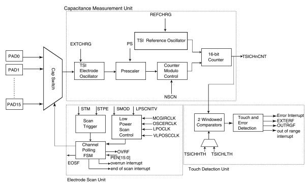
Figure 52-3. TSI block diagram
