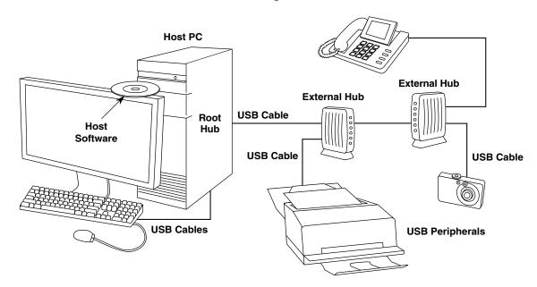
Figure 42-1. Example USB 2.0 system configuration
