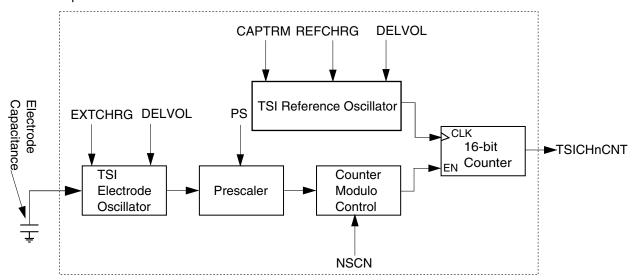
Figure 52-2. TSI capacitance measurement unit block diagram
