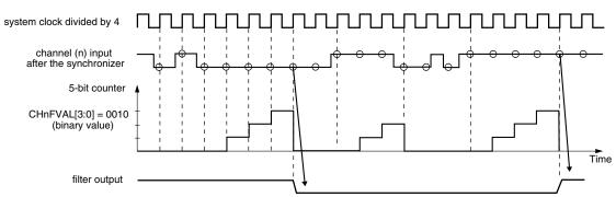
Figure 37-177. Channel input filter example
