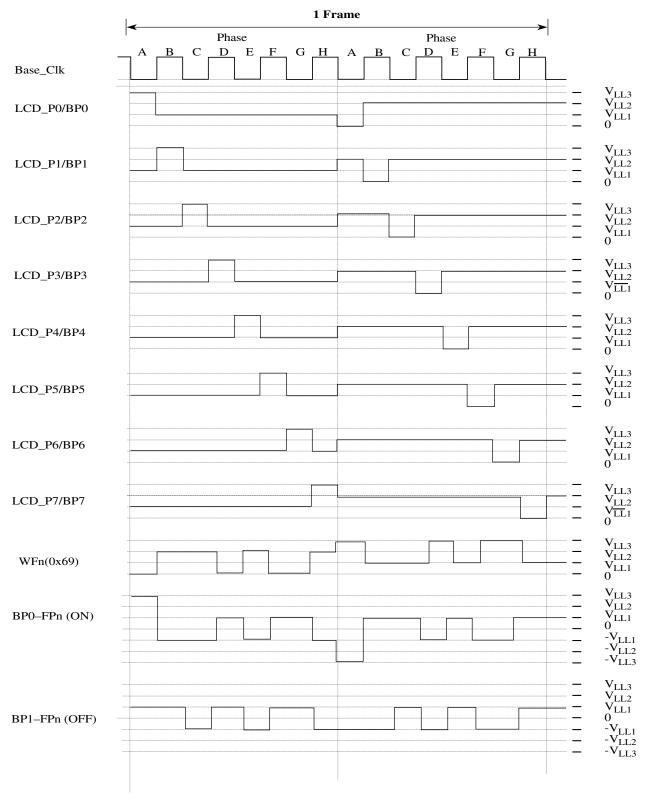
Figure 53-31. 1/8 Duty and 1/3 bias (low-power waveform)
