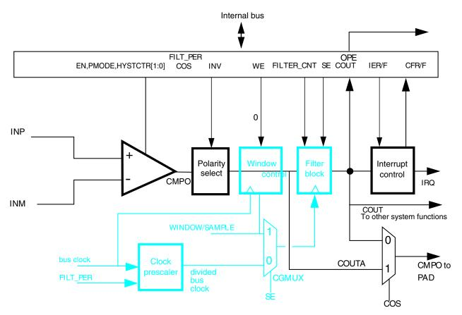
Figure 33-27. Comparator operation in Continuous mode
