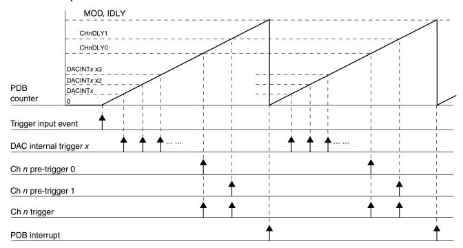
Figure 36-57. PDB ADC triggers and DAC interval triggers use case
