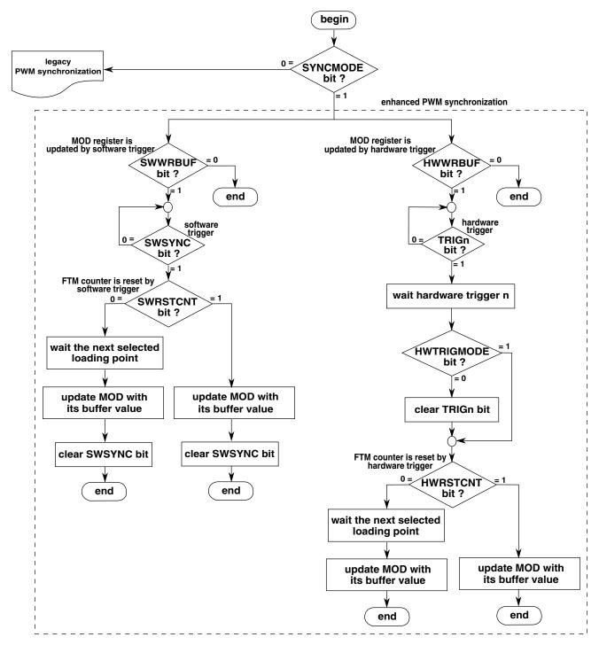
Figure 37-208. MOD register synchronization flowchart
