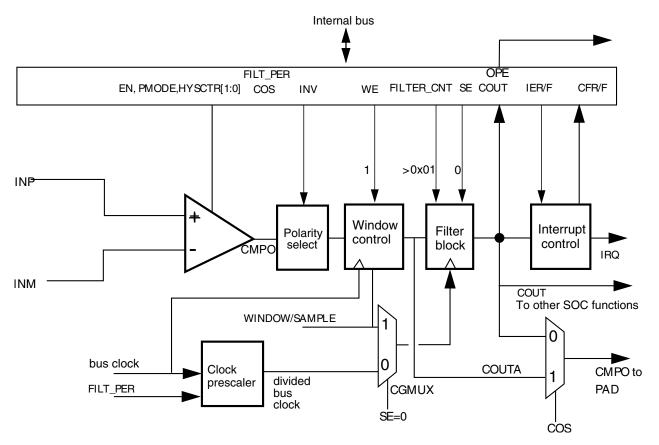
Figure 33-35. Windowed/Filtered mode
