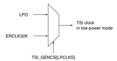
Figure 5-11. TSI low-power clock generation
