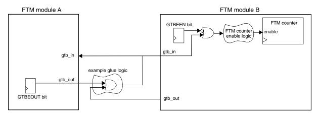
Figure 37-258. Global time base (GTB) block diagram
