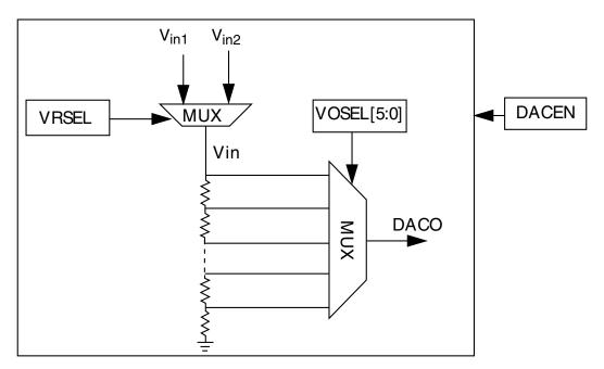
Figure 33-36. 6-bit DAC block diagram
