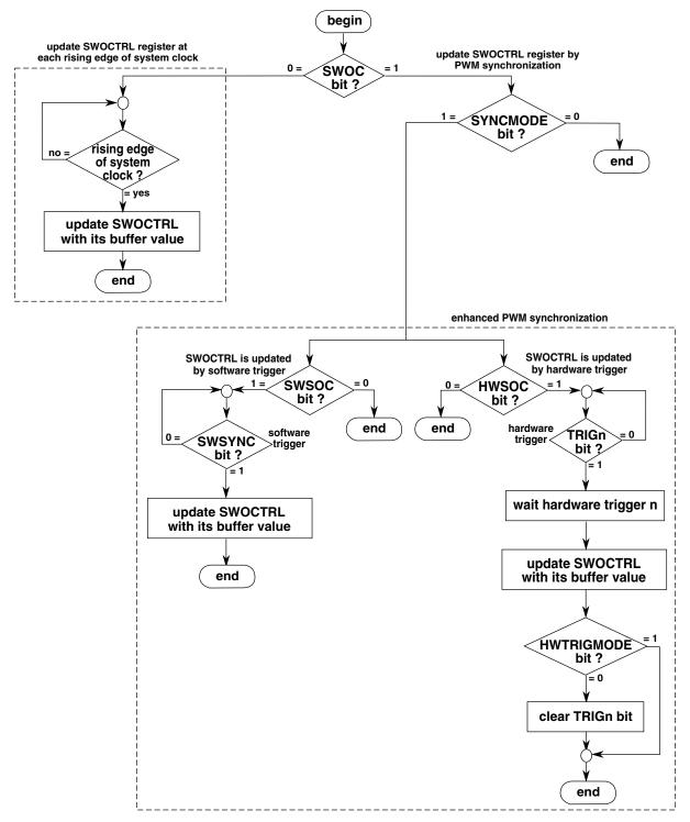
Figure 37-219. SWOCTRL register synchronization flowchart
