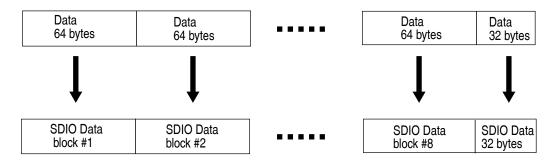
Eight 64 byte blocks are sent in Block transfer mode and the remainder 32 bytes are sent in Byte Transfer mode
