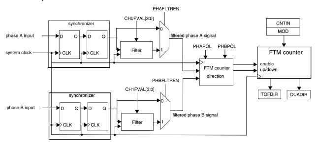
Figure 37-250. Quadrature Decoder block diagram
