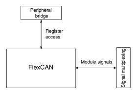
Figure 3-54. CAN configuration
