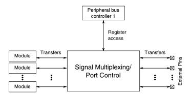
Figure 10-1. Signal multiplexing integration
