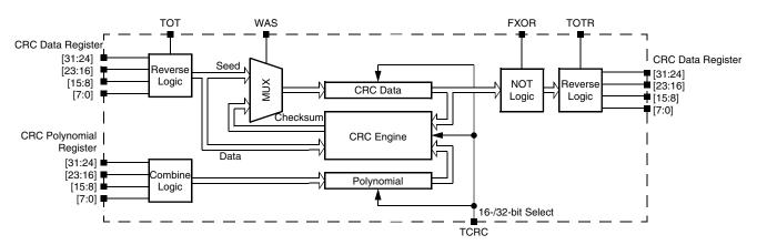
Figure 31-1. Programmable cyclic redundancy check (CRC) block diagram
