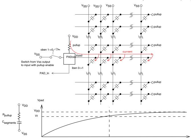
Figure 53-33. Pullup fault detect in connection/segment normal case
