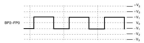
Figure 53-42. "e" segment voltage waveform
