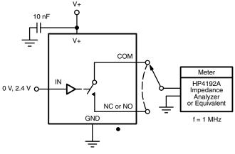
Figure 5. Channel Off/On Capacitance
