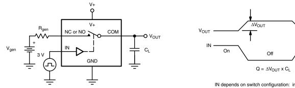
IN depends on switch configuration: input polarity determined by sense of switch.
