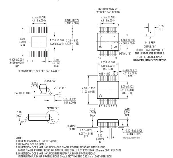
LEAD COPLANARITY (BOTTOM OF LEADS AFTER FORMING) SHALL BE 0.102mm (.004") MAX
