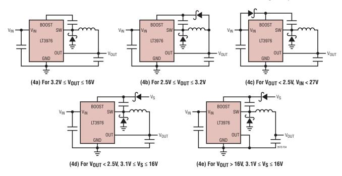
Figure 4. Five Circuits for Generating the Boost Voltage
