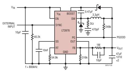
Figure 12b. Fault Tolerant for  $V_{OUT} < 27V$  (Note: For  $V_{OUT} < 3V$  External Boost Schottky Diode Should Be Connected to the Input)
