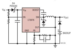
Figure 9. Diode D4 Prevents a Shorted Input from Discharging a Backup Battery Tied to the Output. It Also Protects the Circuit from a Reversed Input. The LT3976 Runs Only When the Input Is Present
