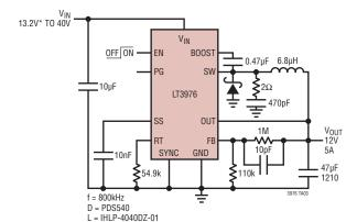
MINIMUM V<sub>IN</sub> CAN BE LOWERED WITH ADDITIONAL INPUT AND OUTPUT CAPACITANCE.
