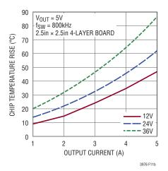
Figure 11b. Temperature Rise of the LT3976 in a  $5\mbox{V}_{OUT}$  Application
