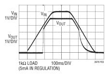
Figure 3. V<sub>IN</sub> to V<sub>OUT</sub> Performance
