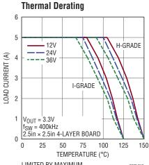
LIMITED BY MAXIMUM 3976 G10 JUNCTION TEMPERATURE  $\Theta_{JA} = 40^{\circ} \text{C/W}$
