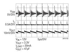
Figure 2. Burst Mode Operation
