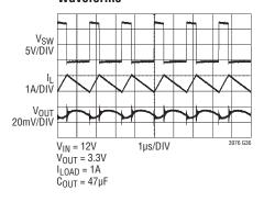
**Dropout Switching Waveforms**
