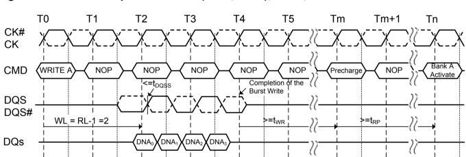
Figure 25. Burst write operation: RL=3 (AL=0, CL=3), WL=2, BL=4
