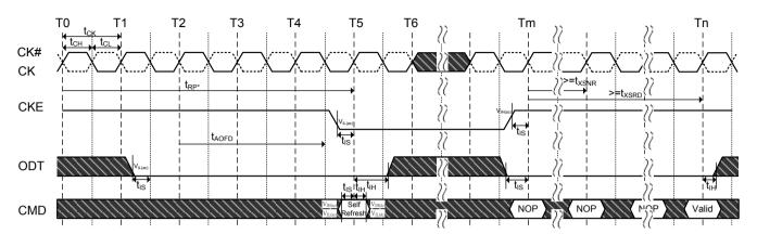
NOTE 1 Device must be in the "All banks idle" state prior to entering Self Refresh mode. NOTE 2 ODT must be turned off  $t_{AOFD}$  before entering Self Refresh mode, and can be turned on again when  $t_{XSRD}$  timing is satisfied.
