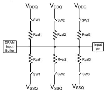
Switch (sw1, sw2, sw3) is enabled by ODT pin. Selection among sw1, sw2, and sw3 is determined by "Rtt (nominal)" in EMR. Termination included on all DQs, DM, DQS, DQS# pins
