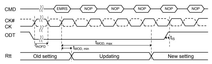
NOTE 1: To prevent any impedance glitch on the channel, the following conditions must be met: - t<sub>AOFD</sub> must be met before issuing the EMRS command.
