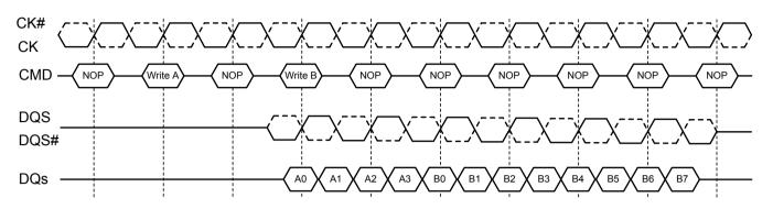
NOTE 1: Write burst interrupt function is only allowed on burst of 8. Burst interrupt of 4 is prohibited.
