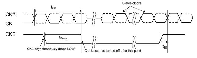
Figure 57. Clock frequency change in precharge power down mode
