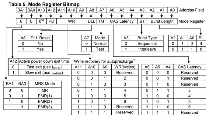
**NOTE 1:** For DDR2-667/800, WR min is determined by  $t_{CK}$  (avg) max and WR max is determined by  $t_{CK}$ (avg) min. WR [cycles] = RU { $t_{WR}$ [ns]/ $t_{CK}$ (avg)[ns]}, where RU stands for round up. The mode register must be programmed to this value. This is also used with  $t_{RP}$  to determine  $t_{DAL}$ .
