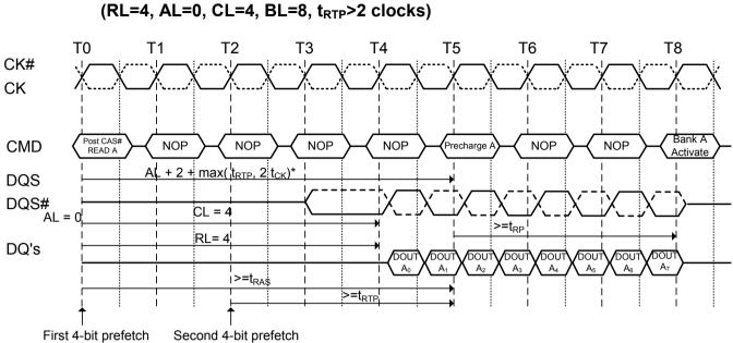
Figure 34. Burst read operation followed by precharge: (RL=4, AL=0, CL=4, BL=8, t<sub>RTP</sub>>2 clocks)
