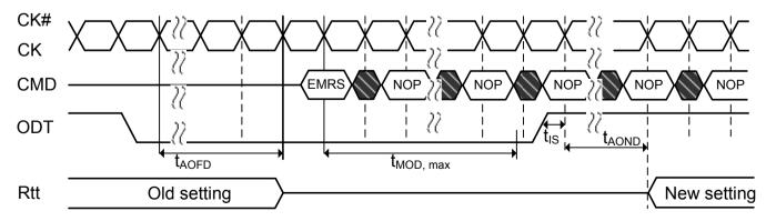
Figure 9. ODT update delay timing- $t_{MOD}$ , as measured from outside
