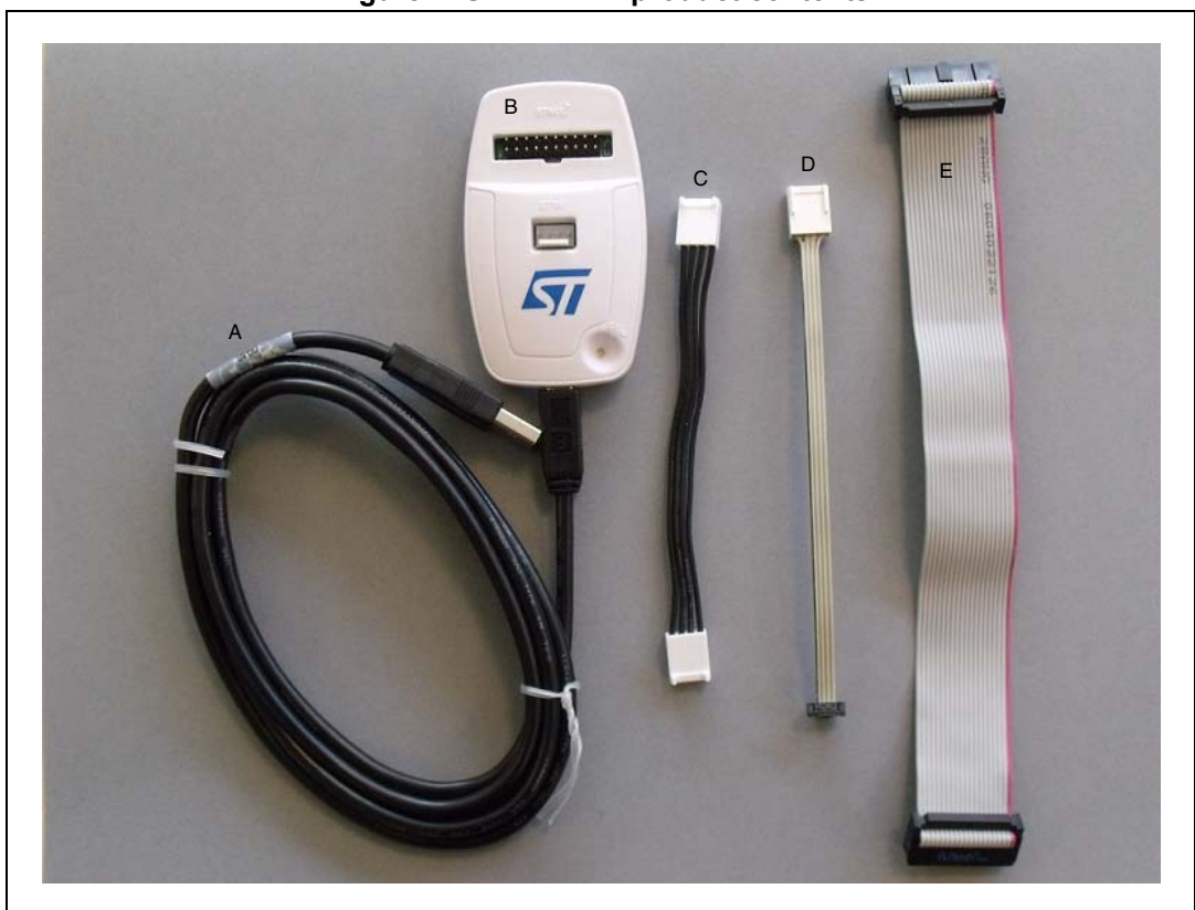
Figure 2. ST-LINK/V2 product contents
