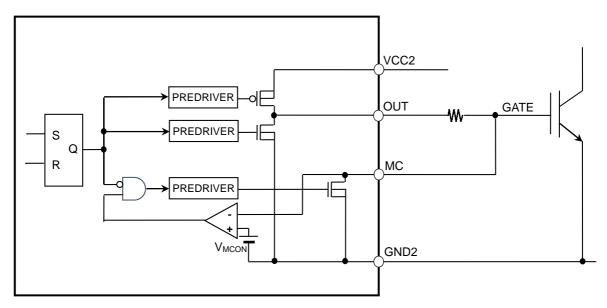
Figure 3. Block diagram of Miller Clamp function.
