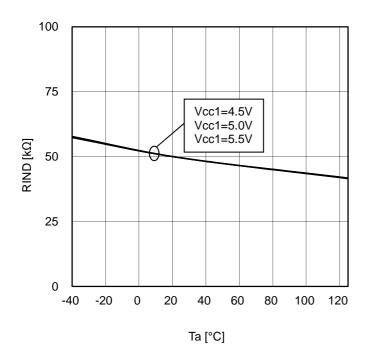
Figure 21. Logic Pull-down Resistance
