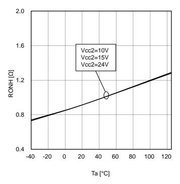
Figure 23. OUT ON Resistance (Source)
