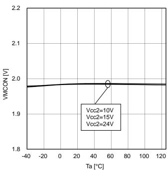
Figure 30. MC ON Threshold Voltage
