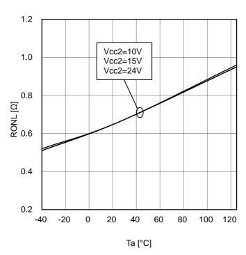
Figure 24. OUT ON Resistance (Sink)
