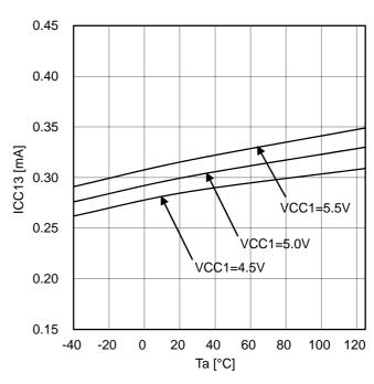
Figure 14. Input Side Circuit Current 3 (at INA=20kHz, Duty=50%)
