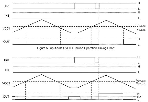
Figure 6. Output-side UVLO Function Operation Timing Chart
