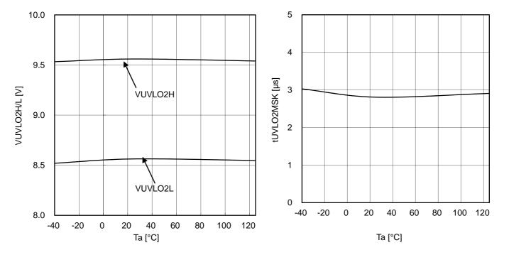
Figure 33. Output Side UVLO ON/OFF voltage
