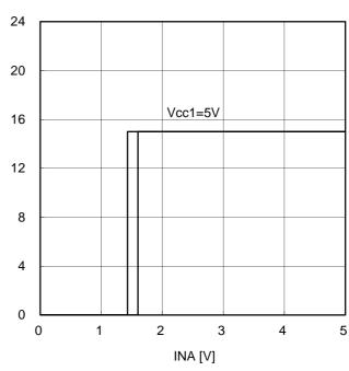
Figure 20. OUT vs Logic (INA) Input Voltage (VCC1=5V, VCC2=15V, Ta=25°C)
