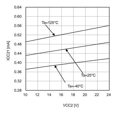
Figure 15. Output Side Circuit Current 1 (at OUT=L)
