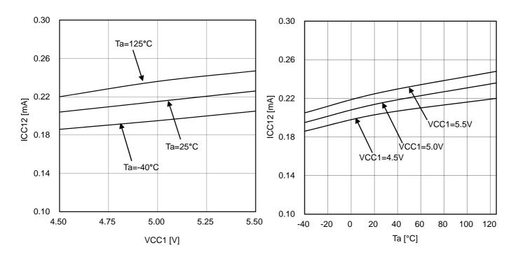
Figure 11. input Side Circuit Current 2 (at INA=10kHz, Duty=50%)
