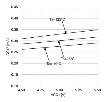
Figure 13. Input Side Circuit Current 3 (at INA=20kHz, Duty=50%)
