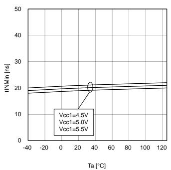
Figure 22. Logic (INA) Input Minimum Pulse Width
