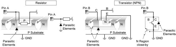
Figure 43. Example of IC structure
