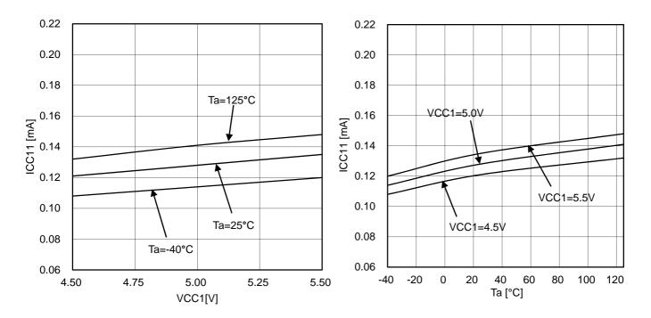
Figure 9. Input Side Circuit Current 1
