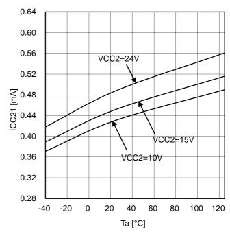
Figure 16. Output Side Circuit Current 1 (at OUT=L)
