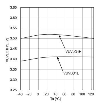
Figure 31. Input Side UVLO ON/OFF Voltage
