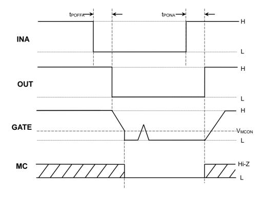
Figure 4. Timing chart of Miller Clamp function
