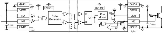
Figure 1. Application Circuits (IGBT Gate Driver)
