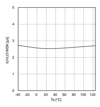
Figure 32. Input Side UVLO Mask Time
