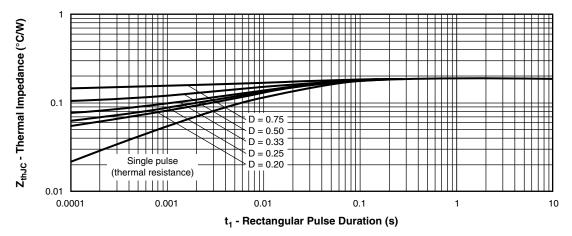
Fig. 4 - Maximum Thermal Impedance  $Z_{\text{thJC}}$  Characteristics, Per Leg
