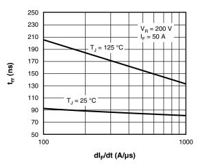
Fig. 7 - Typical Reverse Recovery Time vs. dl<sub>F</sub>/dt, Per Leg
