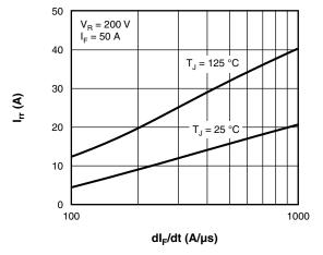
Fig. 9 - Typical Reverse Recovery Current vs. dl<sub>F</sub>/dt, Per Leg
