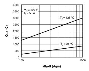
Fig. 8 - Typical Reverse Recovery Charge vs. dl<sub>F</sub>/dt, Per Leg
