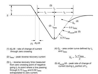
Fig. 11 - Reverse Recovery Waveform and Definitions
