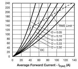
Fig. 6 - Forward Power Loss Characteristics (Per Leg)
