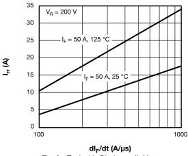
Fig. 9 - Typical Irr Diode vs. dI<sub>F</sub>/dt
