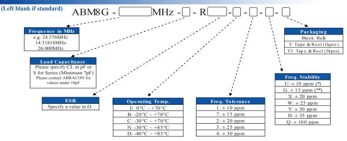
(\*) -10°C to +60°C only. Contact ABRACON for tighter freq. stability. (\*\*) -10°C to +60°C option E,B,C,N only
