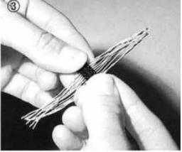
3. Assemble two protectors and temporarily attach to the holder.
