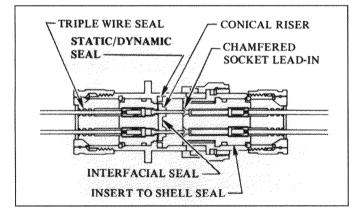
In addition to individual contact sealing, these connectors incorporate additional protective seals to assure sealing against environmental extremes: interfacial compression seal, peripheral static/dynamic shell-to-shell seal, insert-to-shell seal, and redundant rear wire seals.
