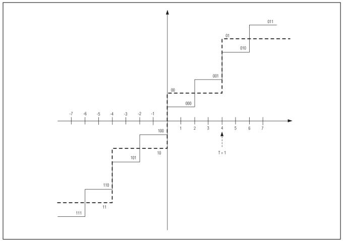
Figure 2. ADC Quantization Levels for 2- and 3-Bit Cases
