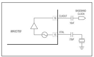
Figure 1. Schematic of the Crystal Oscillator in the MAX2679 EV Kit
