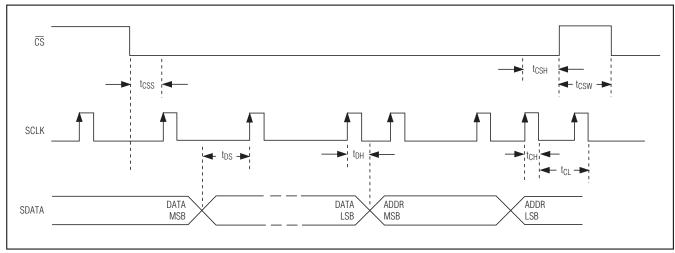
Figure 4. 3-Wire Timing Diagram
