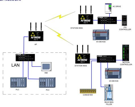
In station WDS mode, the 702-W can be connected to a remote wired Ethernet switch with multiple devices connected to the switch.
