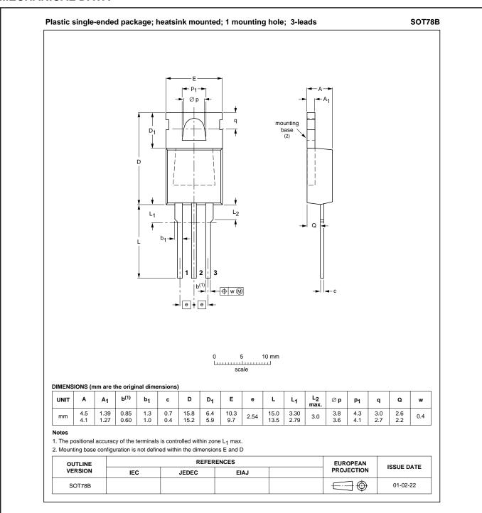
Fig.2. SOT78B (TO220AB) package<sup>1</sup>, pin 2 connected to mounting base.
