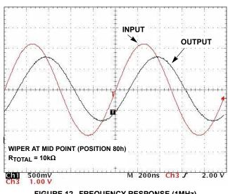
FIGURE 12. FREQUENCY RESPONSE (1MHz)
