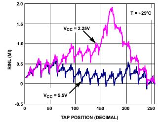
FIGURE 8. INL vs TAP POSITION IN RHEOSTAT MODE FOR 10 k\Omega (W)
