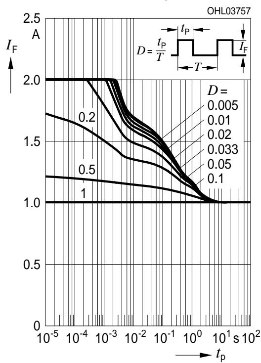
**Zulässige Impulsbelastbarkeit  $I_F = f(t_p)$** **Permissible Pulse Handling Capability**Duty cycle  $D$  = parameter,  $T_S = 85$  °C
