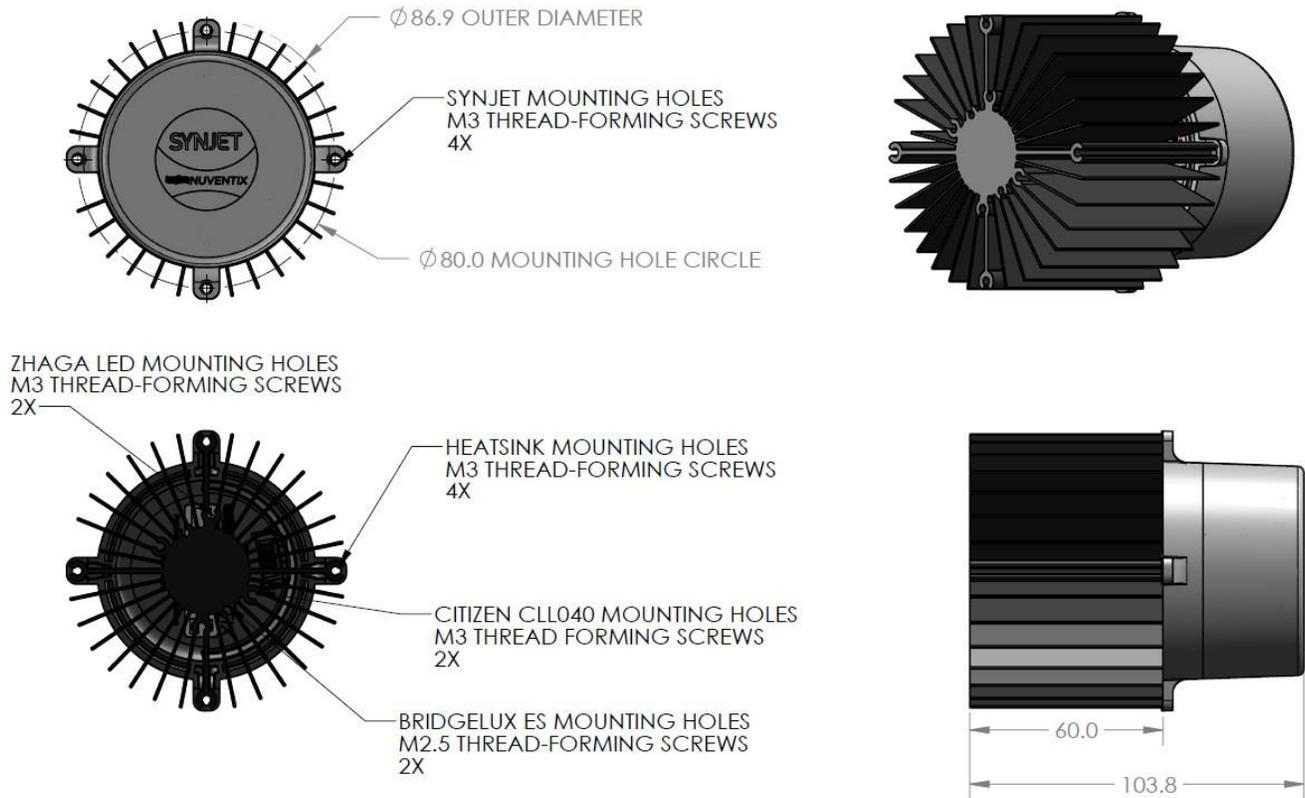
NOTE: DIN 7500 TYPE THREAD-FORMING SCREWS ARE RECOMMENDED FOR ALL MOUNTING HOLE BOSSES
