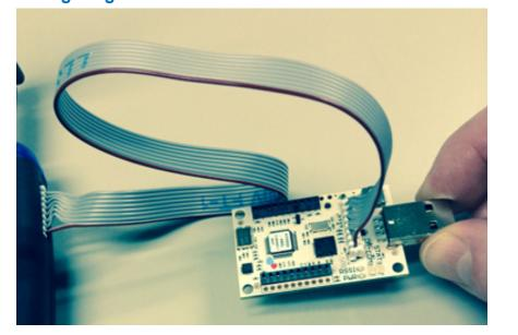
If you want to modify the device settings or reprogram the device, you must order a Micro Developer Kit (MDK), model: MTMDK-ST-MDOT (pictured above), which is sold separately. (Alternatively, a UDK2 can also work. Refer to .net link under **More Information** section.) For programming instructions, visit the mbed.org site: http://developer.mbed.org/getting-started/
