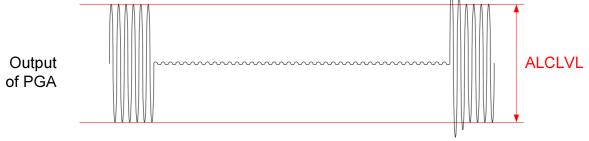
Figure 18 Noise Gate Operation
