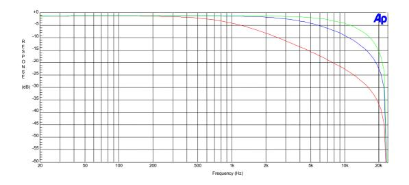
Figure 39 ADC Low Pass Filter Responses (48kHz); fc= 1kHz, 5kHz, 10kHz
