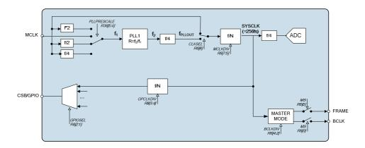
Figure 24 PLL and Clock Select Circuit
