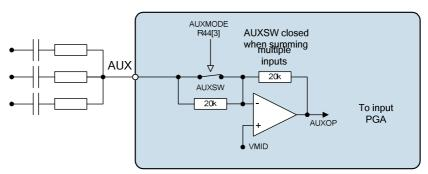
Figure 7 Auxiliary Input Circuit
