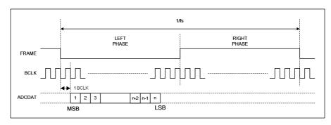
Figure 21 I<sup>2</sup>S Audio Interface (assuming n-bit word length)
