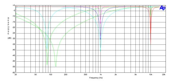
Figure 38 ADC Notch Filter Responses (48kHz); fc=100Hz, 1kHz, 10kHz; fb = 100Hz, 600Hz, 2kHz
