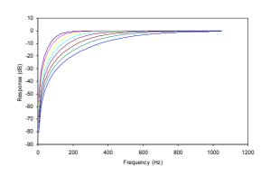
Figure 36 ADC High Pass Filter Responses (24kHz), HPFAPP=1, all cut-off settings shown.
