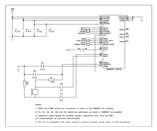
Figure 41 Recommended External Components
