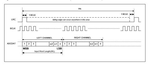
Figure 23 DSP/PCM Mode Audio Interface (Mode B, FRAMEP=1)
