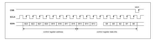
Figure 28 3-Wire Serial Control Interface
