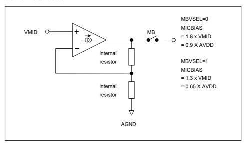
Figure 9 Microphone Bias Schematic
