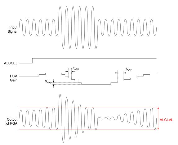
Figure 12 ALC Normal Mode Operation
