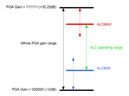
Figure 14 ALC Min/Max Gain
