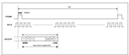
Figure 22 DSP/PCM Mode Audio Interface (Mode A, FRAMEP=0)
