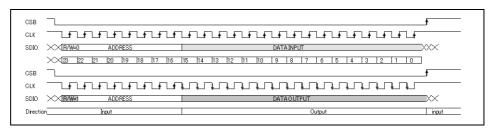
Figure 29 Alternative 3-Wire Serial Control Timing
