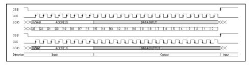
Figure 30 Alternative 3-Wire Serial Control Timing
