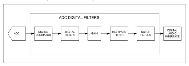
Figure 10 ADC Digital Filter Path
