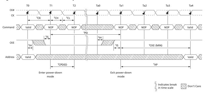
Figure 96: Precharge Power-Down (Fast-Exit Mode) Entry and Exit
