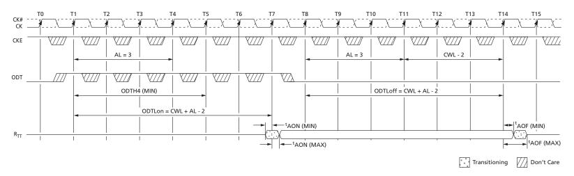
Note: 1. AL = 3; CWL = 5; ODTLon = WL = 6.0; ODTLoff = WL - 2 = 6. R<sub>TT,nom</sub> is enabled.
