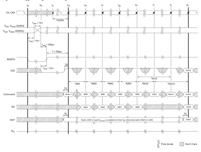
Note: 1. From time point Td until Tk, NOP or DES commands must be applied between MRS and ZQCL commands.
