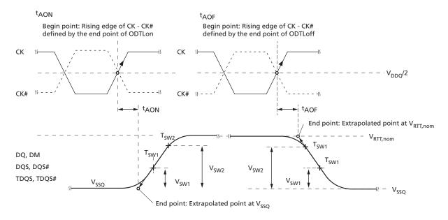
Figure 23: <sup>t</sup>AONPD and <sup>t</sup>AOFPD Definitions
