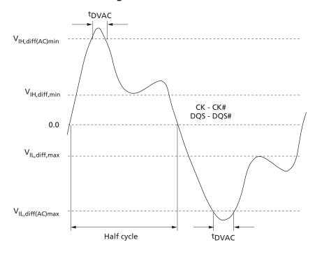
Table 27: DDR3L 1.35V - Minimum Required Time <sup>t</sup>DVAC for CK/CK#, DQS/DQS# Differential for AC Ringback
