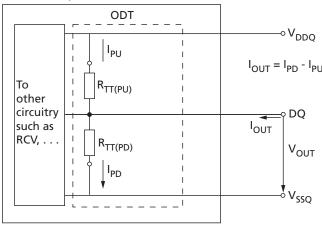
**Table 30: On-Die Termination DC Electrical Characteristics**
