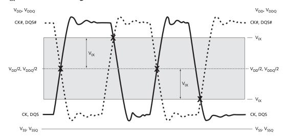
Figure 16: Single-Ended Requirements for Differential Signals
