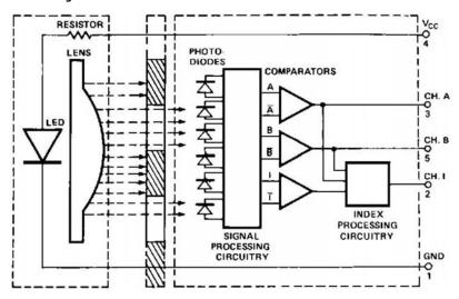
Note: Circuitry for CH I is only for HEDS-5540, 5640 and HEDM 5540 Three Channel Encoder
