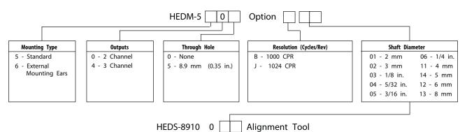
(Included with each order of HEDM-550X/560X two channel encoders and HEDM-554X three Channel encoders)
