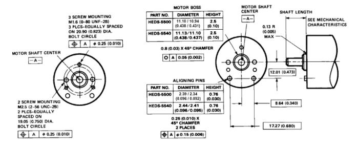
Figure 2. Mounting Holes.
