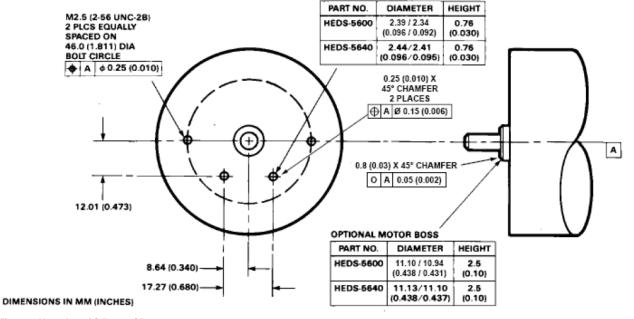
Figure 4. Mounting with External Ears.
