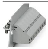
Panel feed-through terminal block, Connection method: Screw connection, Bolt connection, Load current: 150 A, Cross section: 16 mm² - 50 mm², AWG 6 - 1/0, Connection direction of the conductor to plug-in direction: 90 °, Width: 18.8 mm, Color: gray
