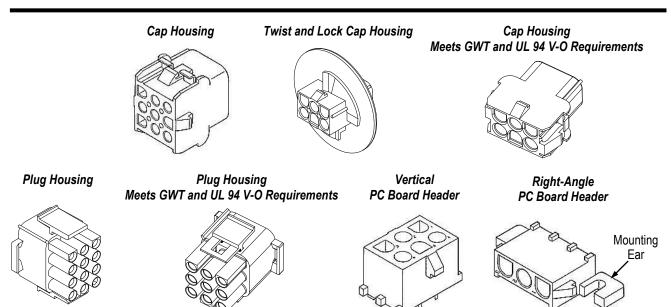
GWT is the glow wire test required by IEC/EN 60335-1
