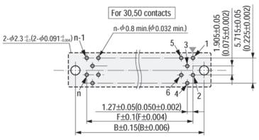
All=Polarity identification Recommended PCB Thickness t=1.6±0.19(0.063±0.007) "n" is number of contacts.
