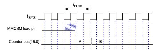
Figure G-41 MMCSM Load Pin to Counter Bus Reload Timing Diagram
