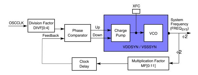
Figure 8-3 System PLL Block Diagram
