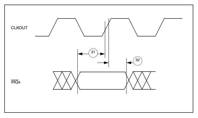
Figure G-18 Interrupt Detection Timing for External Level Sensitive Lines
