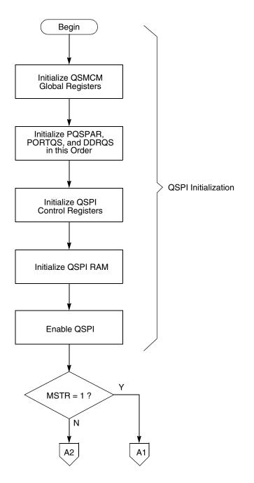
Figure 14-6 Flowchart of QSPI Initialization Operation
