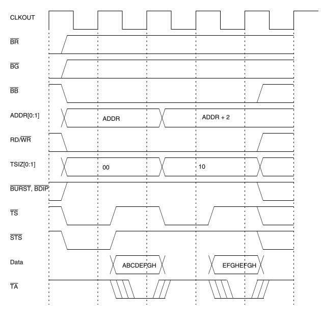
Figure 9-10 Single Beat 32-Bit Data Write Cycle Timing, 16 Bit-Port Size
