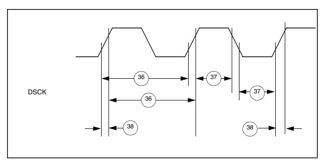
Figure G-20 Debug Port Clock Input Timing
