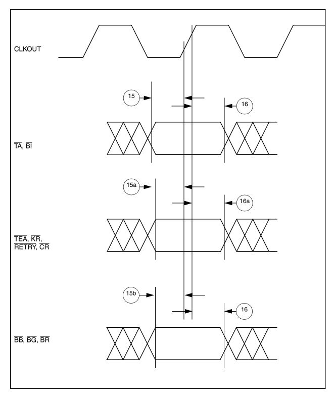
Figure G-5 Synchronous Input Signals Timing
