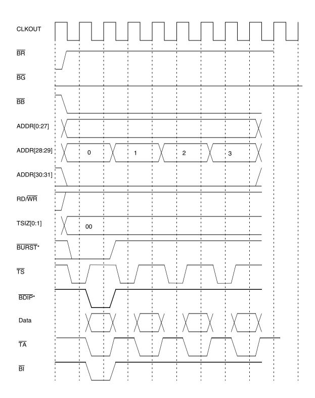
\* BURST and BDIP will be asserted for one cycle if the RCPU core requests a burst, but the USIU splits it into a sequence of normal cycles.
