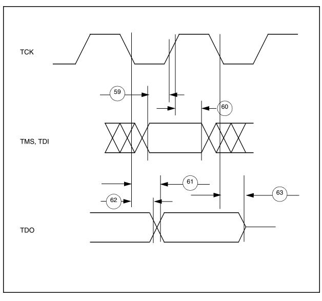
Figure G-26 JTAG — Test Access Port Timing Diagram
