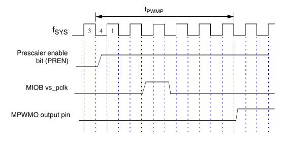
Note:  $F_{SYS}$  is the internal IMB clock for the IMB3 bus.
