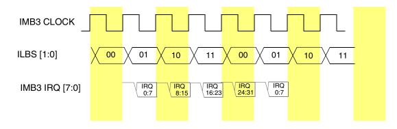
Figure 13-11 Interrupt Levels on IRQ with ILBS
