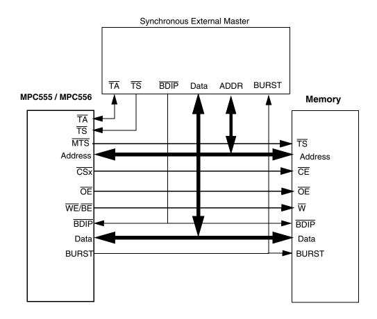
Note that the memory controller's BDIP line is used as a burst\_in\_progress signal.
