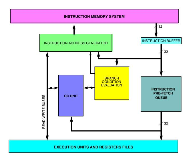
Figure 3-2 Sequencer Data Path
