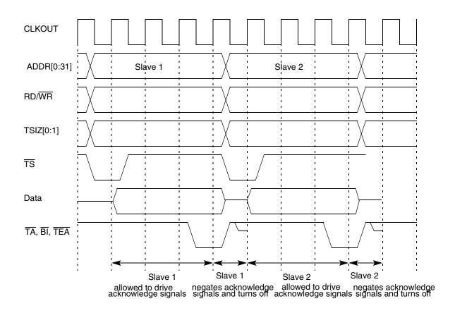
Figure 9-28 Termination Signals Protocol Timing Diagram
