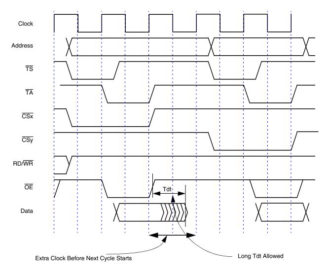
Figure 10-15 Consecutive Accesses (Read After Read From Different Banks, EHTR = 1) **Figure 10-16** shows two consecutive read cycles from the same bank. Even though EHTR = 1, no extra clock cycle is inserted between the memory cycles. (In the case of two consecutive read cycles to the same region, data contention is not a concern.)
