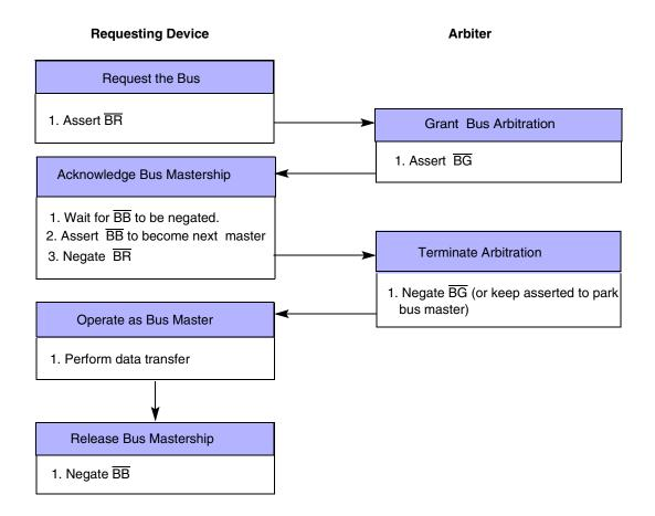
Figure 9-23 Bus Arbitration Flowchart
