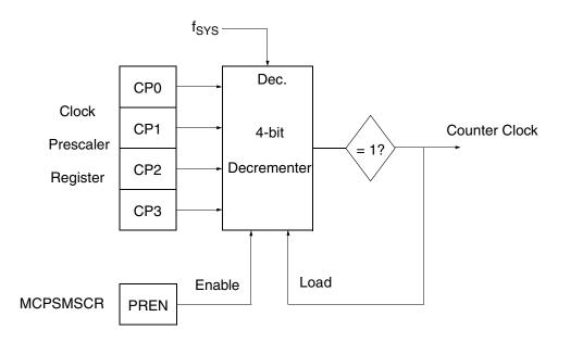
Figure 15-3 MCPSM Block Diagram
