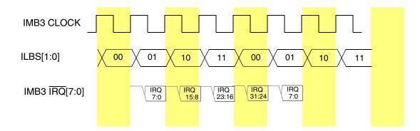
Figure 17-2 TPU3 Interrupt Levels
