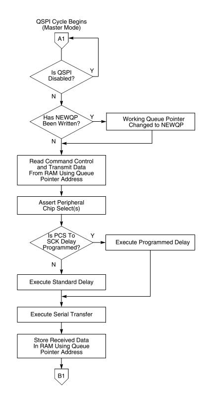
Figure 14-7 Flowchart of QSPI Master Operation (Part 1)
