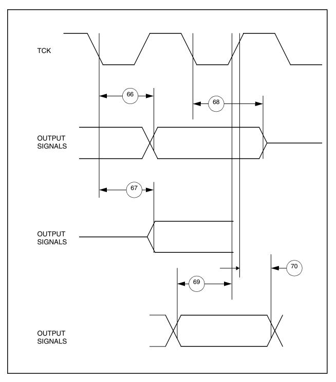
Figure G-28 Boundary Scan (JTAG) Timing Diagram
