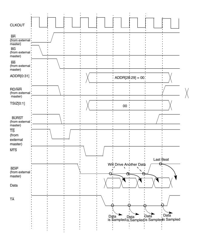
Figure 9-17 Burst-Write Cycle, 32-Bit Port Size, Zero Wait States
