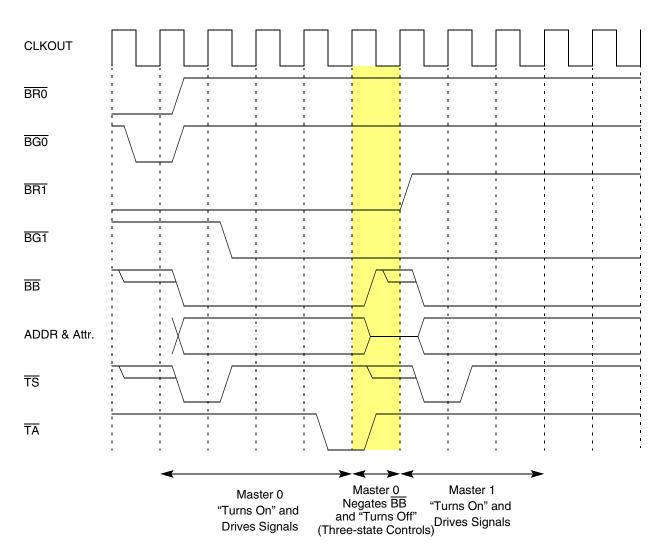
Figure 9-25 Bus Arbitration Timing Diagram
