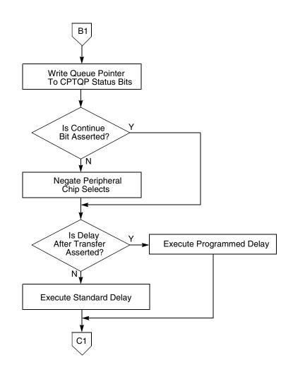
Figure 14-8 Flowchart of QSPI Master Operation (Part 2)
