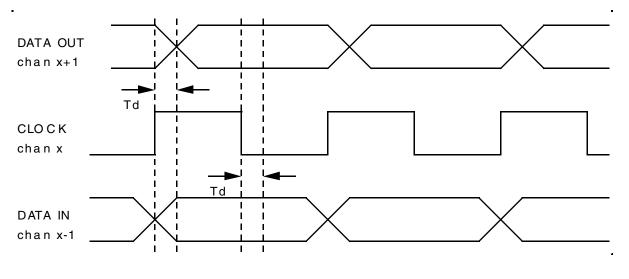
Figure D-31 SIOP Function Data Transition Example
