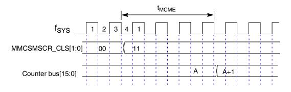
Figure G-43 MMCSM Prescaler Clock Select to Counter Bus Increment Timing Diagram
