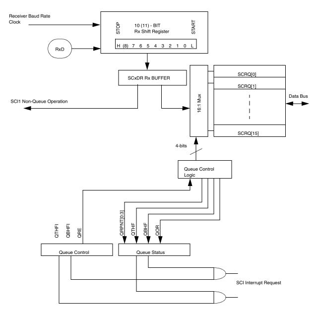
Figure 14-20 Queue Receiver Block Enhancements
