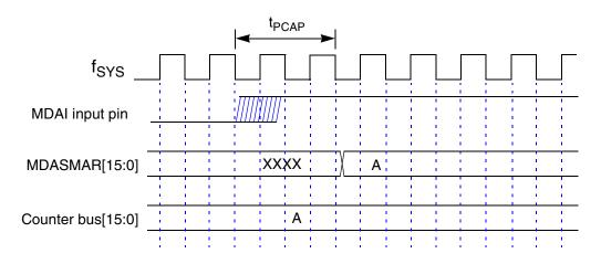
Figure G-45 MDASM Input Pin to Counter Bus Capture Timing Diagram
