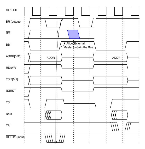
Figure 9-32 Retry Transfer Timing–External Arbiter
