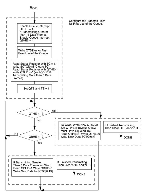
Figure 14-17 Queue Transmit Software Flow
