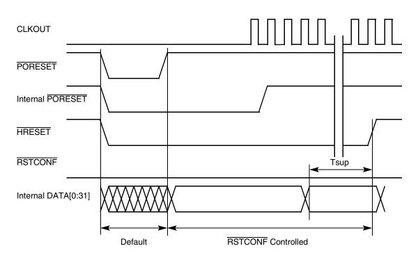
Figure 7-2 to Figure 7-5 provide sample reset configuration timings.
