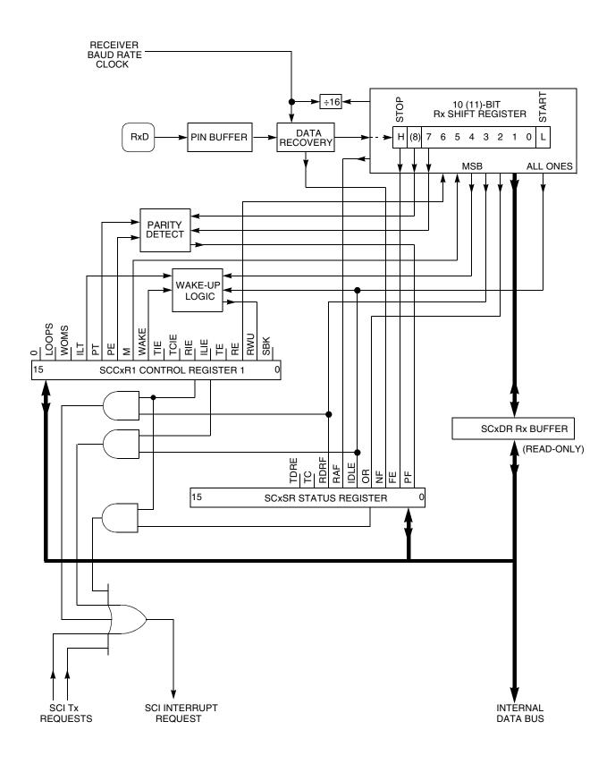
Figure 14-13 SCI Receiver Block Diagram
