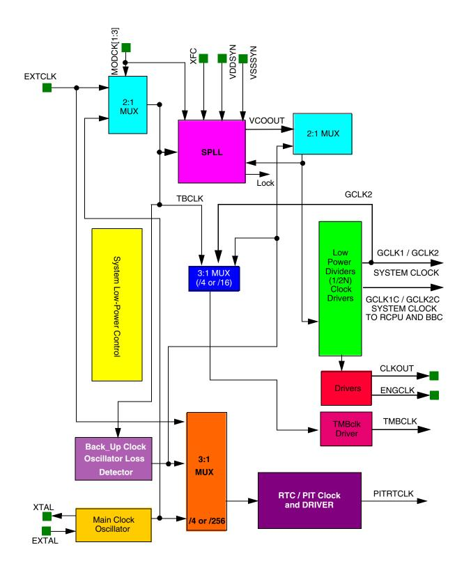
Figure 8-1 Clock Unit Block Diagram
