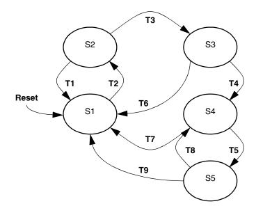
Figure 19-4 Erase State Diagram
