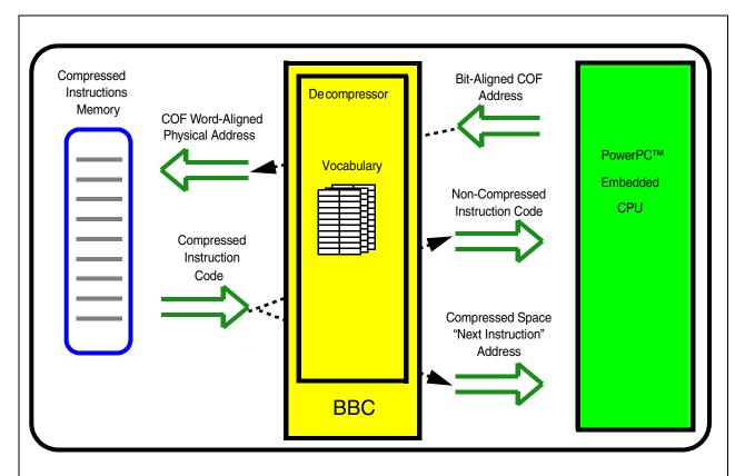
Figure 4-13 Code Decompression Process
