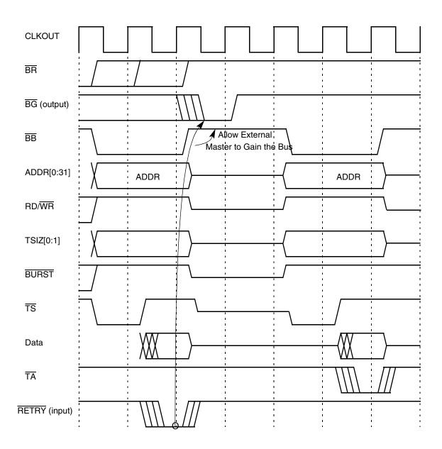
Figure 9-31 Retry Transfer Timing–Internal Arbiter
