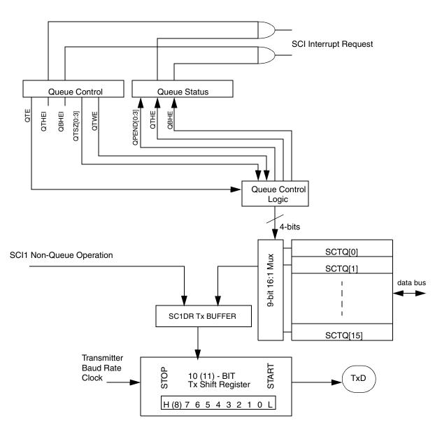
Figure 14-15 Queue Transmitter Block Enhancements
