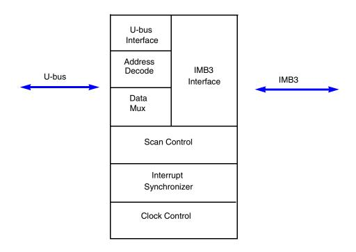
Figure 12-1 UIMB Interface Module Block Diagram
