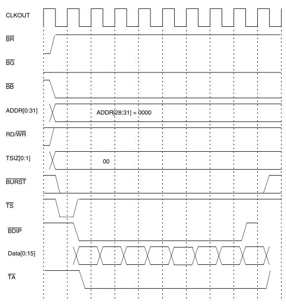
Figure 9-15 Burst-Read Cycle, 16-Bit Port Size
