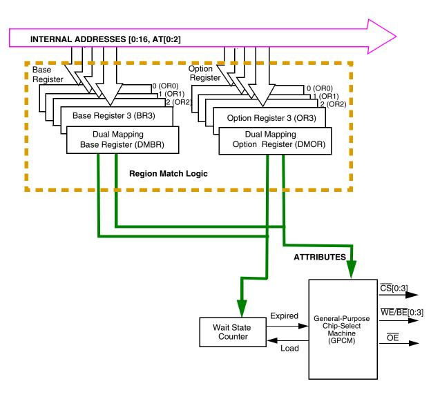
Figure 10-2 Memory Controller Block Diagram
