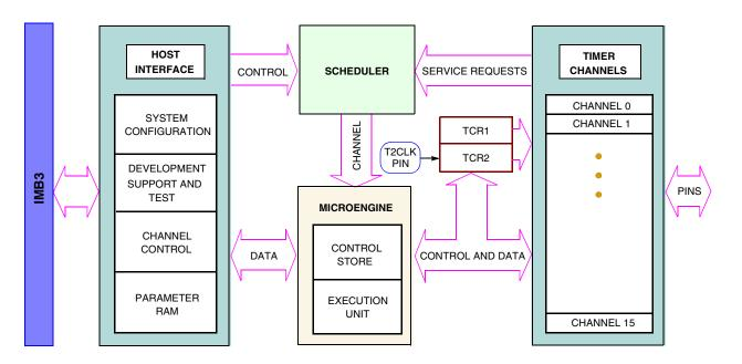
Figure 17-1 TPU3 Block Diagram
