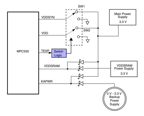
Figure 8-11 External Power Supply Scheme
