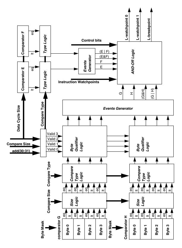
Figure 21-4 Load/Store Support General Structure
