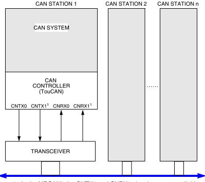
1. In the MPC555, the CNTX1 and CNRX1 signals are not available.
