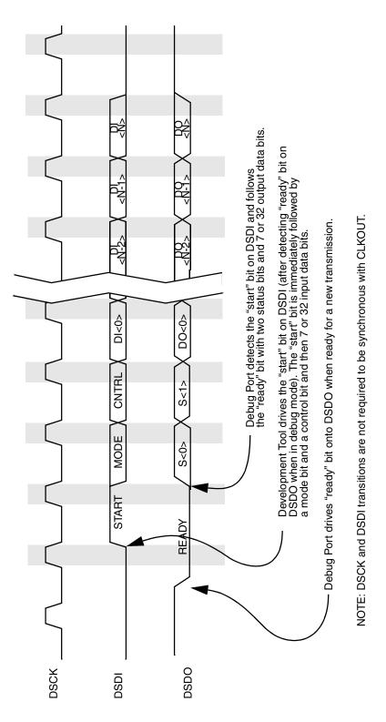
Figure 21-8 Asynchronous Clock Serial Communications
