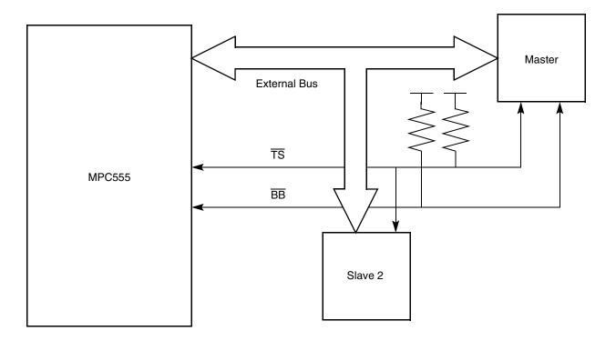
Figure 9-24 Masters Signals Basic Connection
