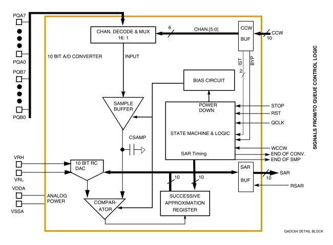
Figure 13-4 QADC64 Module Block Diagram
