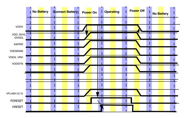
Figure 8-14 Standby and KAPWR, Other Power-On/Off
