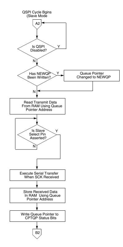
Figure 14-10 Flowchart of QSPI Slave Operation (Part 1)
