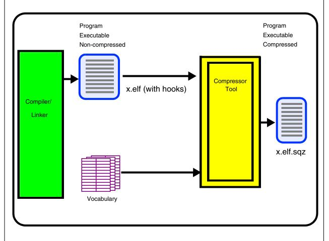
Figure 4-11 Code Compression Process (Phase A)
