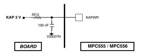
Figure E-4 RC Filter Example
