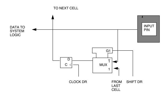
Figure 22-6 Observe-Only Input Pin Cell (I.Obs)
