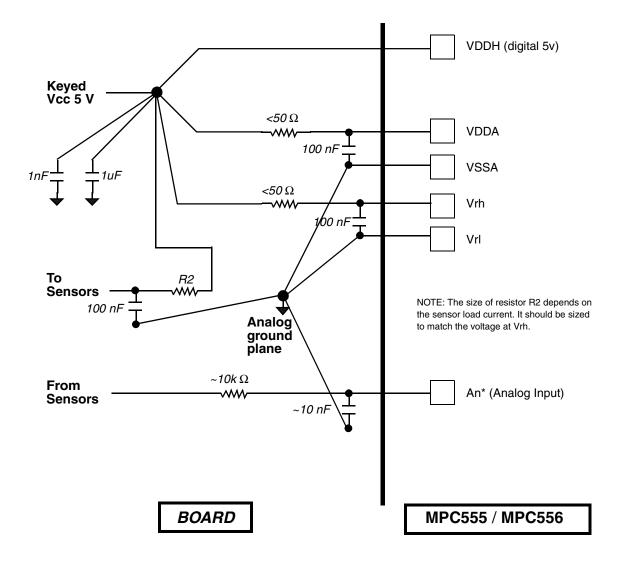
Figure E-2 MPC555 / MPC556 Family Power Distribution Diagram — 5 V and Analog
