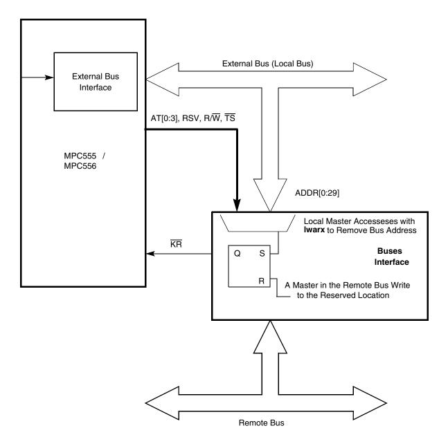
Figure 9-30 Reservation On Multilevel Bus Hierarchy
