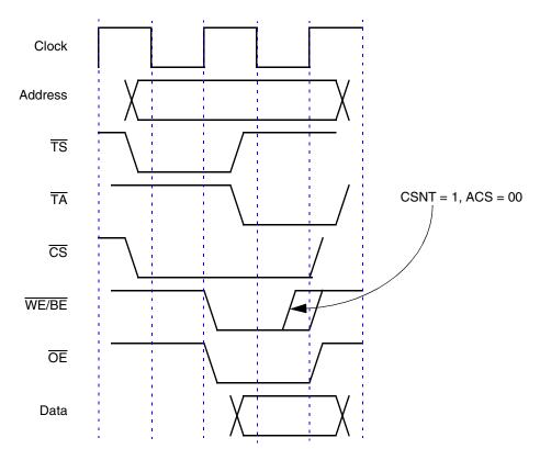
Note: In this and subsequent timing diagrams in this section, the data bus refers to a read cycle. In a write cycle, the data immediately follows  $\overline{TS}$ .
