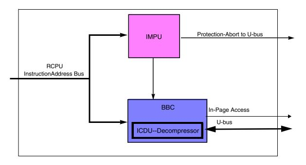
Figure 4-1 Burst Buffer Block Diagram
