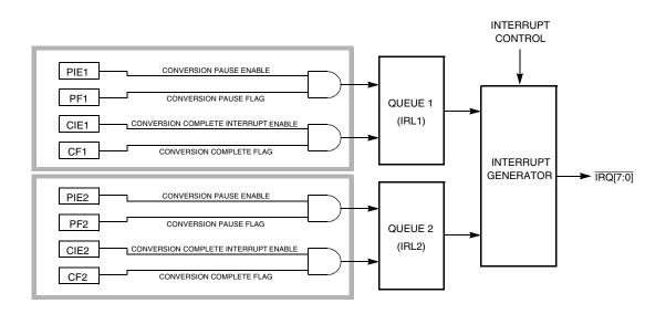
Figure 13-10 QADC64 Interrupt Flow Diagram
