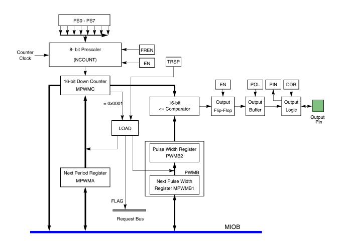
Figure 15-6 MPWMSM Block Diagram
