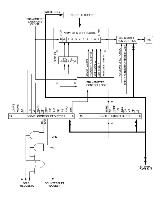
Figure 14-12 SCI Transmitter Block Diagram
