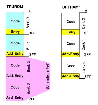
\*The DPTRAM is located at 0x30 2000 until it is switched to emulation mode. In emulation mode, the DPTRAM is accessible by the TPUs only.
