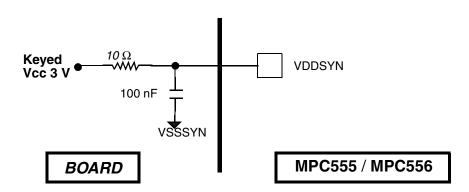
Figure E-6 RC Filter Example
