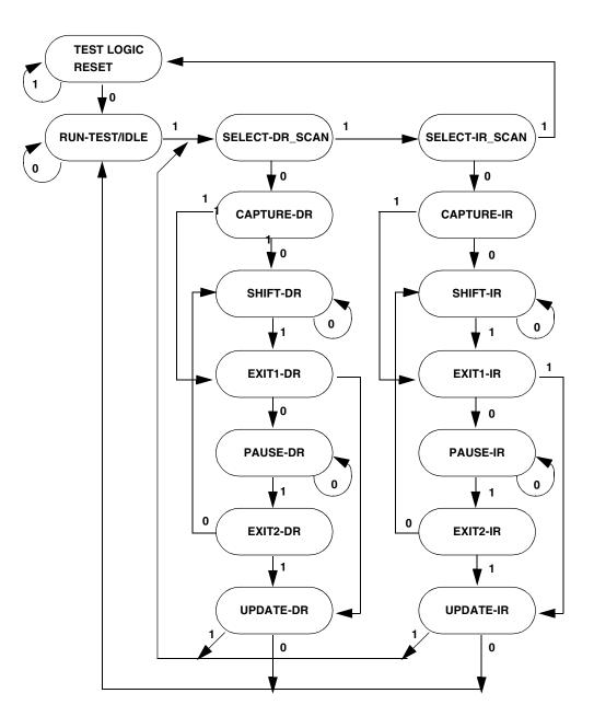
Figure 22-3 TAP Controller State Machine
