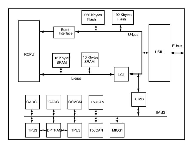
Figure 1-1 MPC555 / MPC556 Block Diagram
