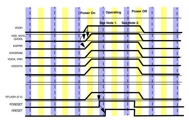
Figure 8-13 No Standby, No KAPWR, All System Power On/Off
