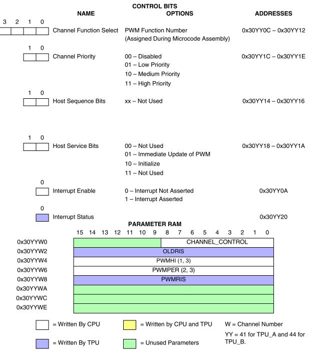
Figure D-23 PWM Parameters
