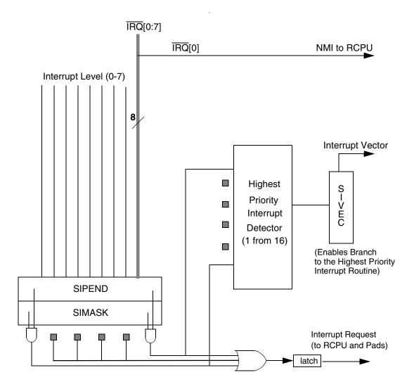
Figure 6-5 MPC555 / MPC556 Interrupt Configuration
