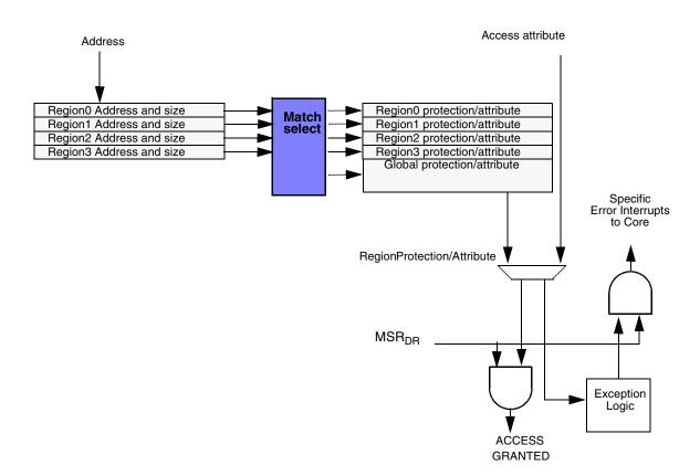
Figure 11-2 DMP Basic Functional Diagram
