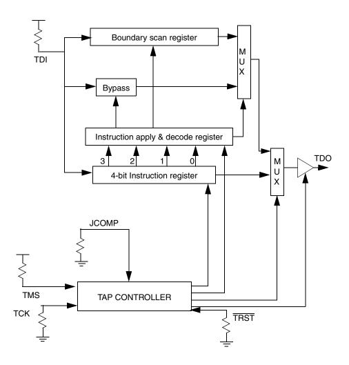
Figure 22-2 Test Logic Block Diagram
