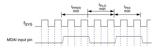
${\rm f}_{\rm SYS}$  is the internal IMB clock for the IMB3 bus.
