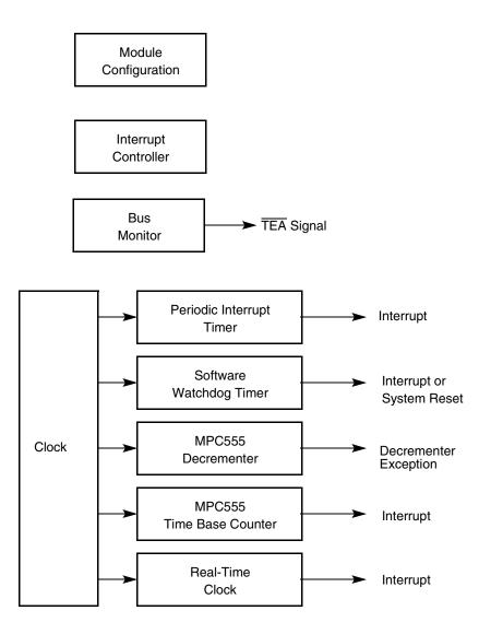
Figure 6-1 System Configuration and Protection Logic
