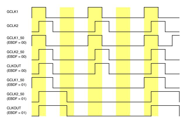
Figure 8-7 Clocks Timing For DFNH = 1 (or DFNL = 0)
