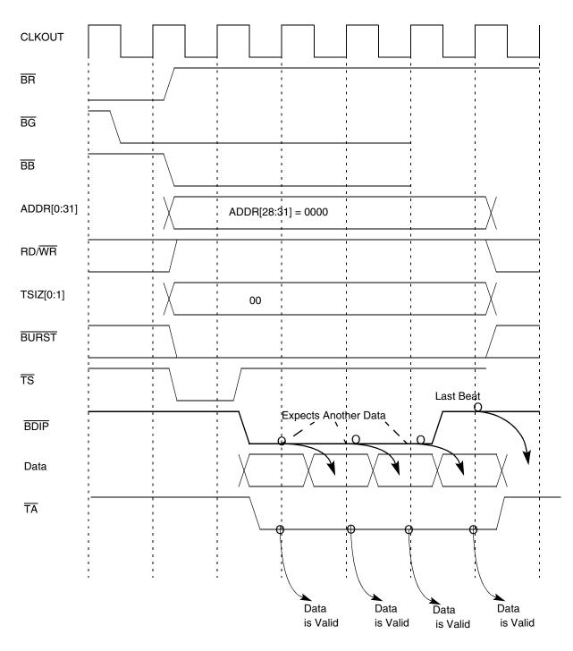
Figure 9-12 Burst-Read Cycle–32-Bit Port Size–Zero Wait State
