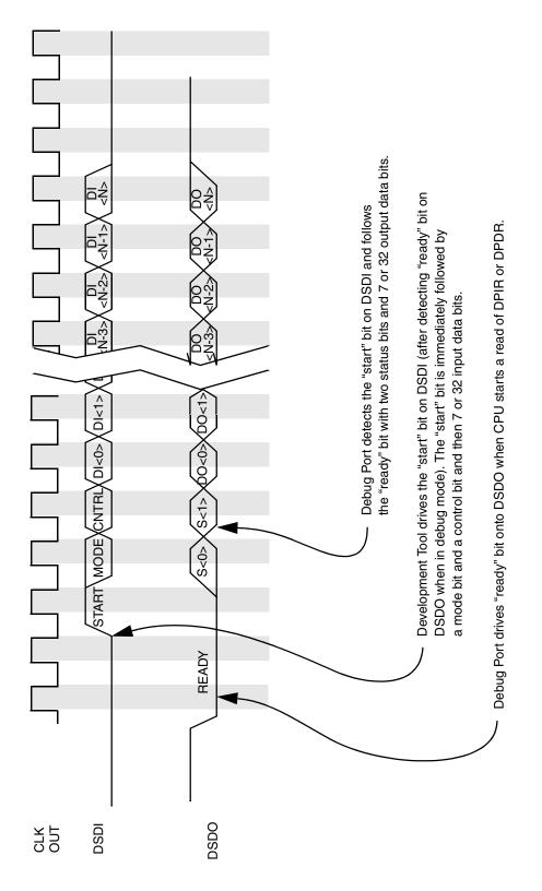
Figure 21-9 Synchronous Self Clock Serial Communication
