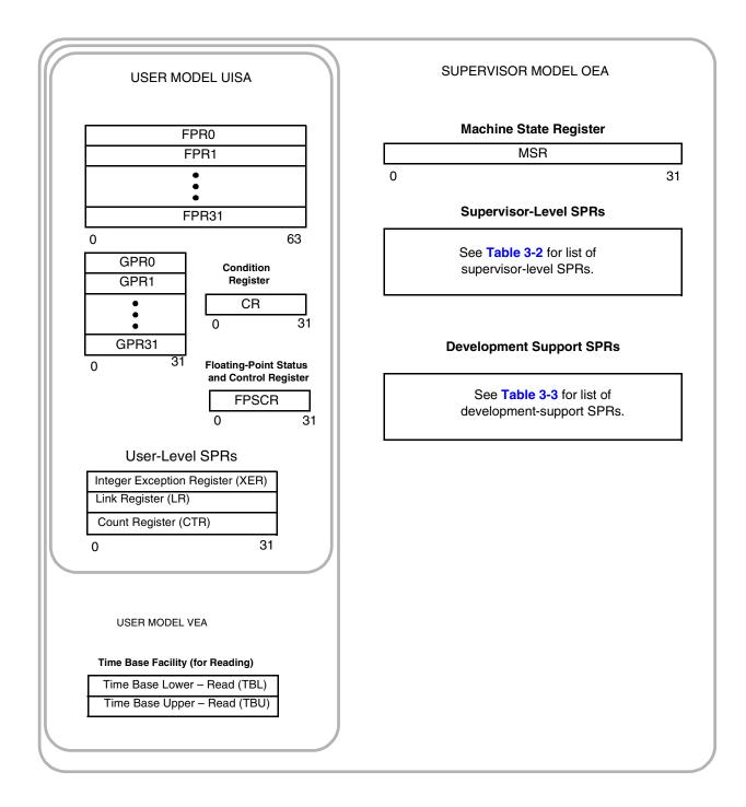
Figure 3-3 RCPU Programming Model
