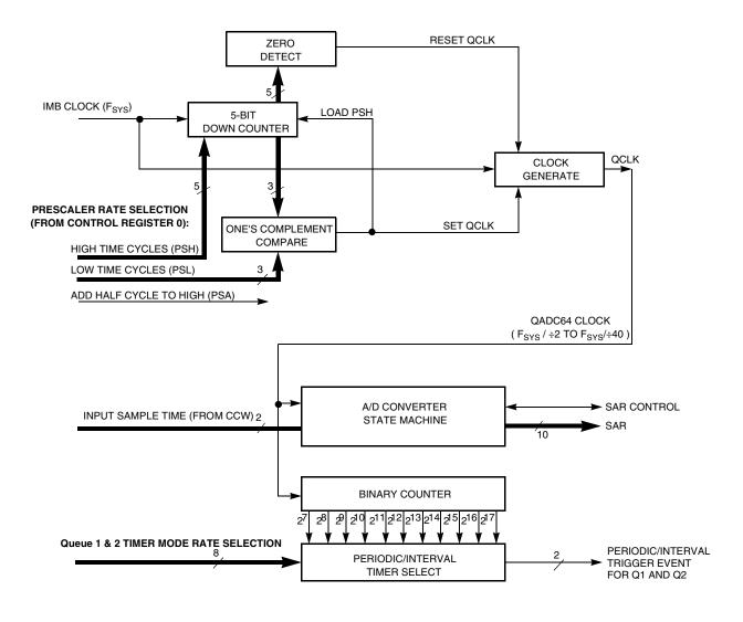
Figure 13-8 QADC64 Clock Subsystem Functions
