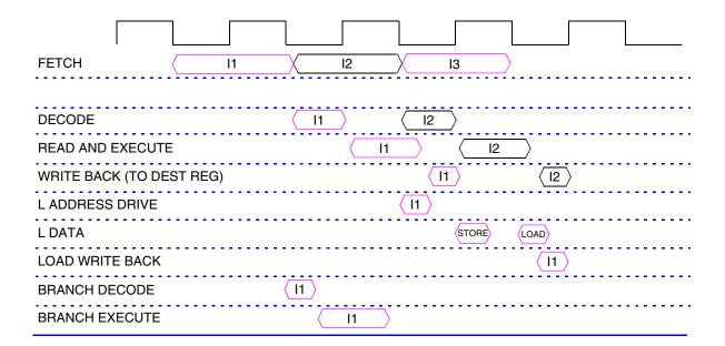
Figure 3-4 shows basic instruction pipeline timing.
