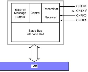
Figure 16-1 shows a block diagram of a TouCAN module.
