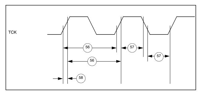
Figure G-25 JTAG Test Clock Input Timing
