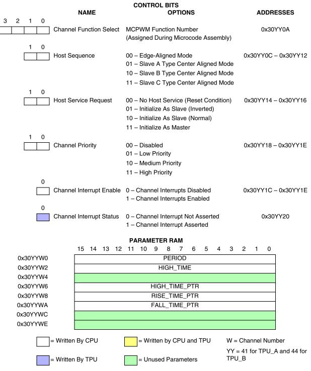
Figure D-14 MCPWM Parameters — Slave Edge-Aligned Mode
