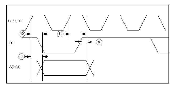
Figure G-11 Address Show Cycle Bus Timing
