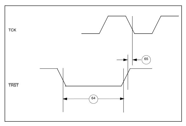
Figure G-27 JTAG — TRST Timing Diagram
