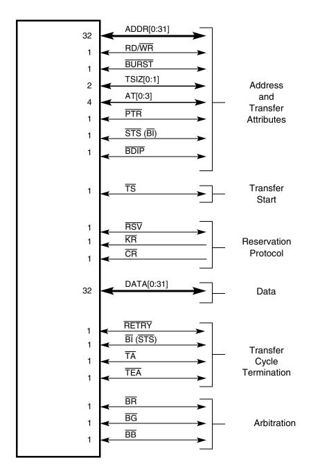
Figure 9-2 MPC555 / MPC556 Bus Signals
