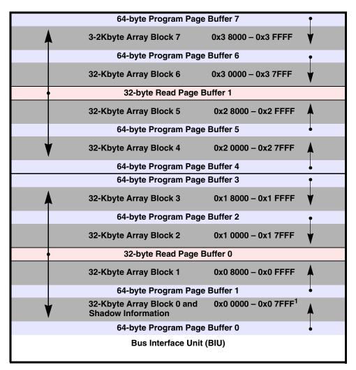
1·If SIE=1, then the shadow row is enabled instead of the flash block. Shadow locations 0x00 to 0x03 are reserved for the Internal Flash Reset Configuration word. Shadow locations 0x04 to 0x0F are Reserved by Motorola for possible future use.
