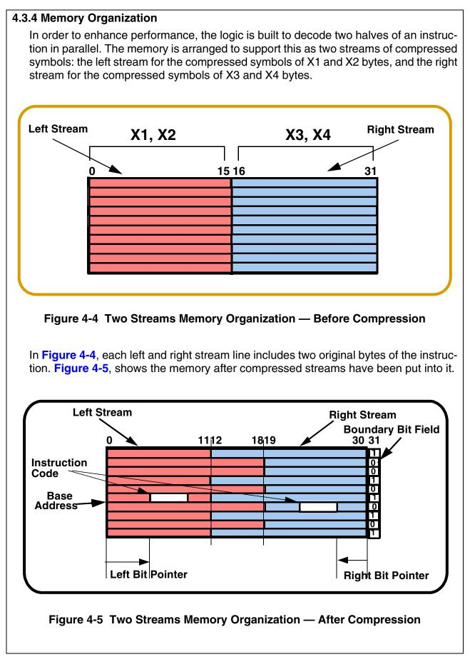
The compiler will set the left and right stream boundary at either bit 12 or bit 19. This will be determined by the most efficient placement of compressed instruction code. The boundary will be placed between bits 11 and 12 if bit 31 is equal to one. The boundary will be placed between bits 18 and 19 if bit 31 is equal to zero. The original right and left streams may span an adjacent base addresses before or after each other. This fact will also determine the placement of the boundary bit field.
