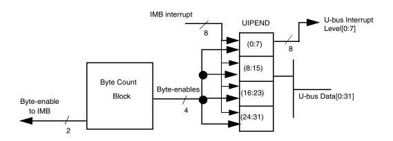
Figure 12-4 Interrupt Synchronizer Signal Flow
