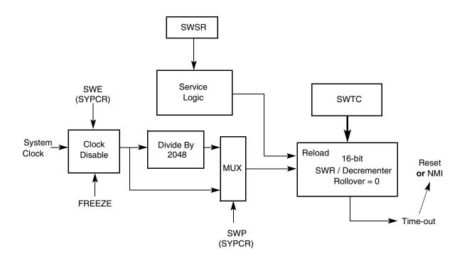
Figure 6-9 SWT Block Diagram
