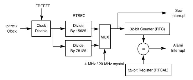
Figure 6-6 RTC Block Diagram
