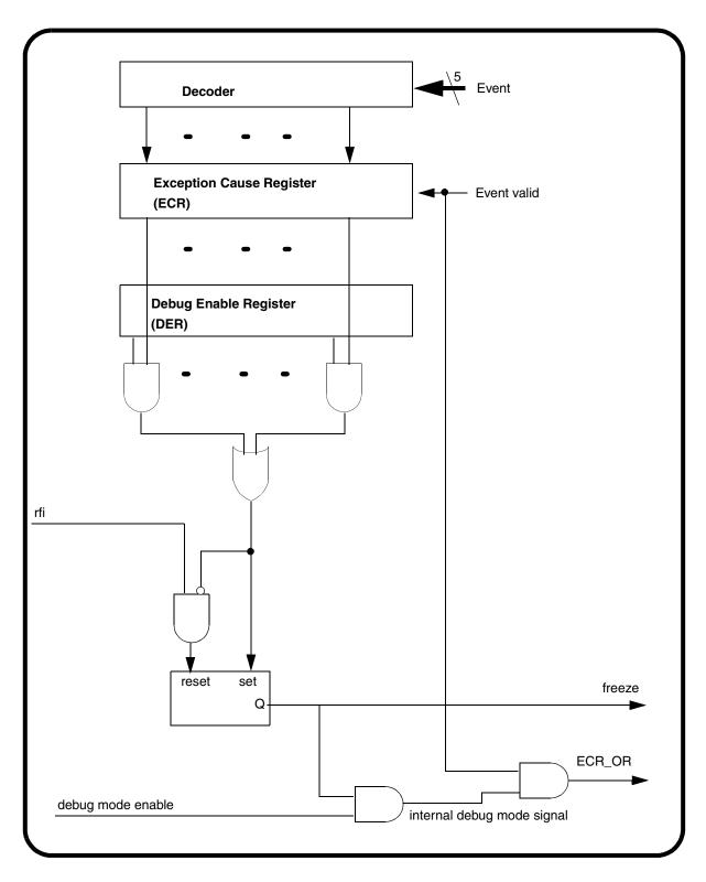
Figure 21-6 Debug Mode Logic
