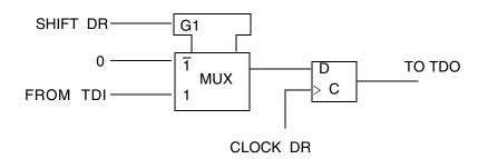
Figure 22-4 Bypass Register
