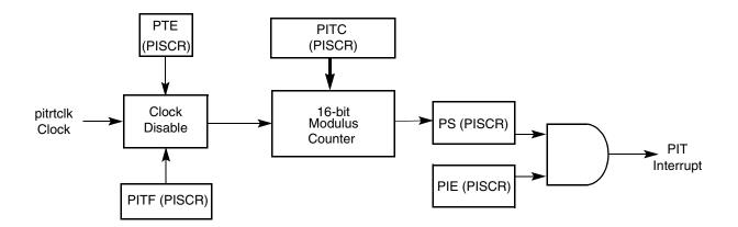
Figure 6-7 PIT Block Diagram
