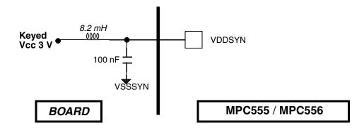
Figure E-7 LC Filter Example (Alternative)
