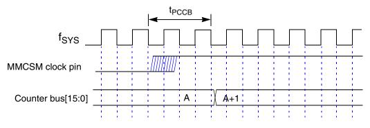
Note:  $F_{SYS}$  is the internal IMB clock for the IMB3 bus.
