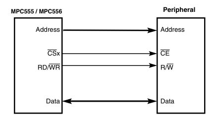
Figure 10-7 Peripheral Devices Interface
