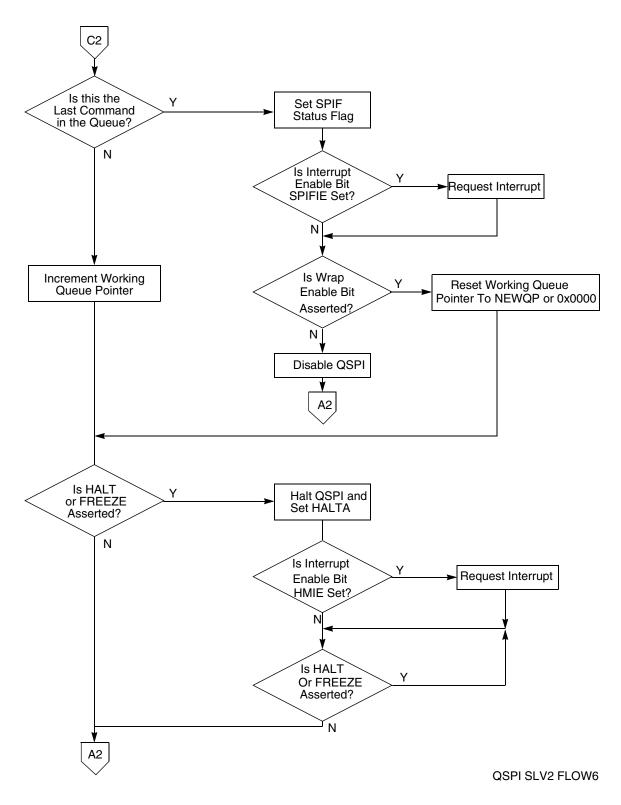
Figure 14-11 Flowchart of QSPI Slave Operation (Part 2)
