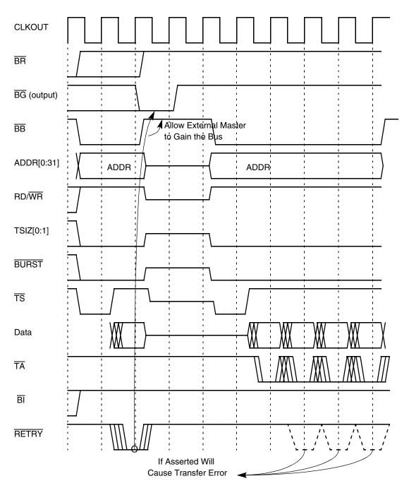
Figure 9-33 Retry On Burst Cycle
