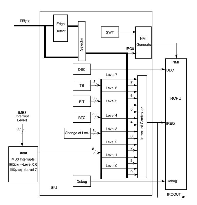
Figure 6-4 MPC555 / MPC556 Interrupt Structure
