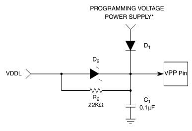
\*The VPP voltage specification is the voltage at the VPP pin, not the input to diode D1.
