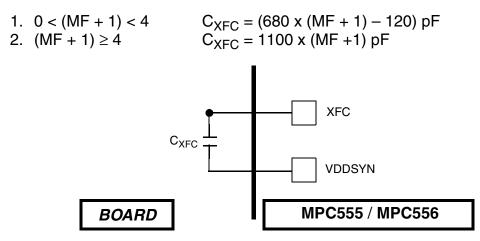
Figure E-8 PLL Off-Chip Capacitor Example
