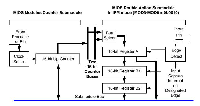
Figure 15-10 MIOS1 Example: Double Capture Period Measurement
