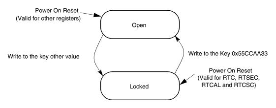
Figure 8-12 Keep Alive Register Key State Diagram
