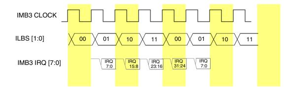
Figure 16-5 Interrupt levels on IRQ with ILBS
