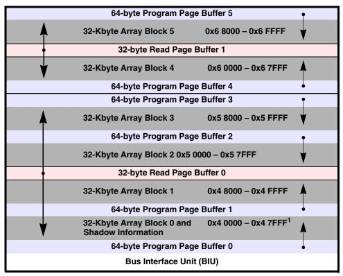
1. If SIE=1, then the shadow row is enabled instead of the flash block. Locations 0x4 00000 to 0x4 000F of the shadow row are Reserved by Motorola for possible future use.
