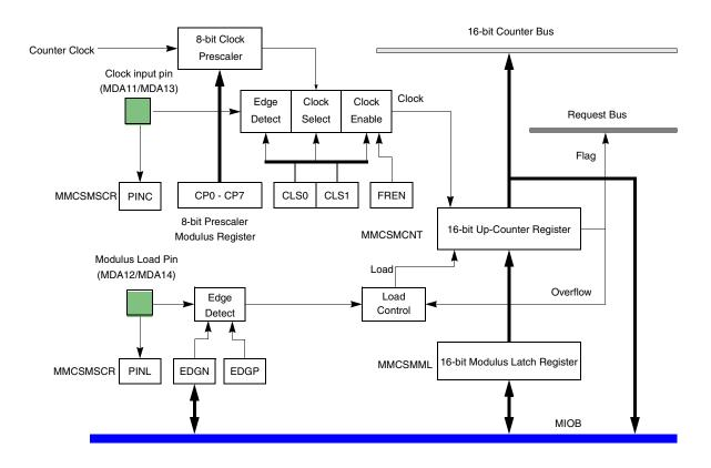
Figure 15-4 MMCSM Block Diagram
