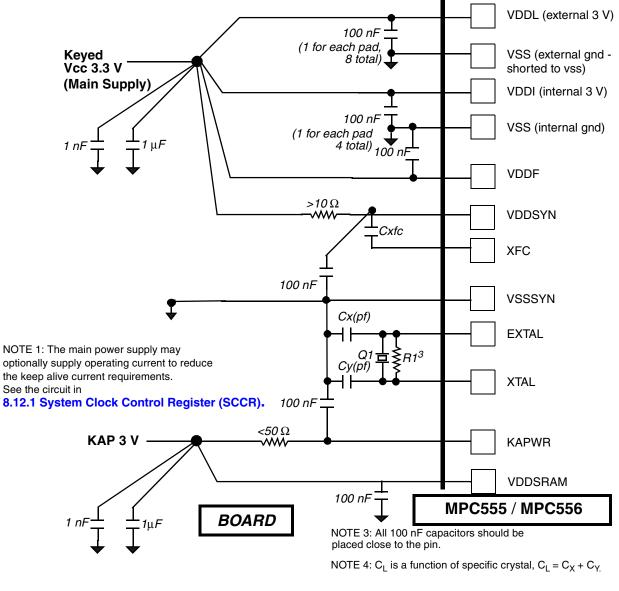
NOTE 2: Resistor  $R_1$  is currently not required. Space should be left on the board to add it in the future if necessary.
