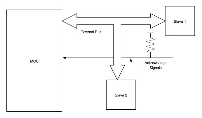
Figure 9-27 Termination Signals Protocol Basic Connection
