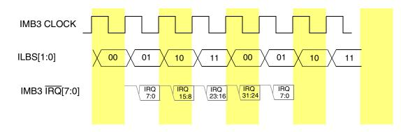
Figure 14-2 QSMCM Interrupt Levels
