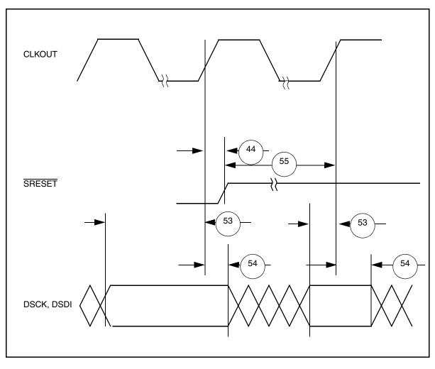
Figure G-24 Reset Timing — Debug Port Configuration
