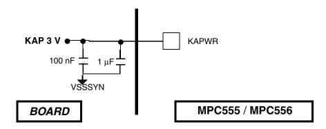
Figure E-5 Bypass Capacitors Example (Alternative)
