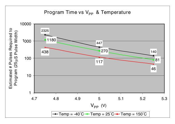
Figure H-1 Typical Program Time vs. V<sub>PP</sub> and Temperature (for CDR1 "Target" Process)
