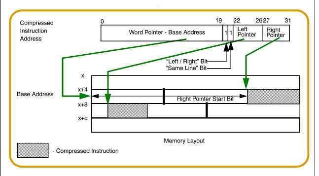
Figure 4-7 Compressed Address Format
