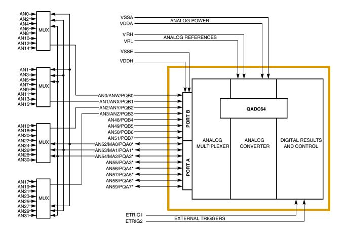
Figure 13-3 Example of External Multiplexing
