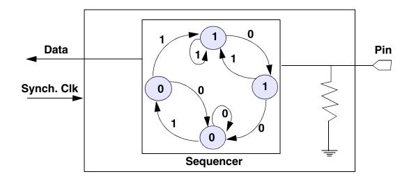
Figure 2-18 EPEE Pad (Type K)
