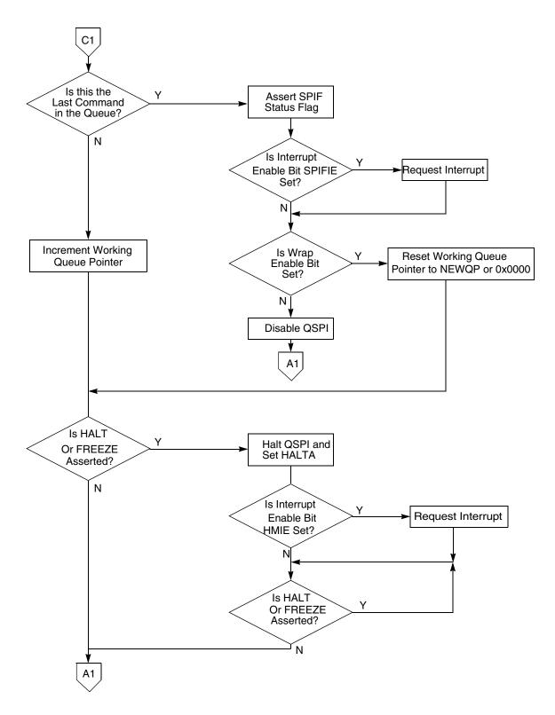
Figure 14-9 Flowchart of QSPI Master Operation (Part 3)
