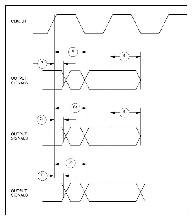
Figure G-3 Synchronous Output Signals Timing
