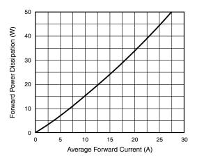
Fig. 3 - Forward Power Dissipation
