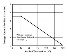
Fig. 2 - Forward Current Derating Curve
