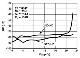
FIGURE 6. 200kHz 2ND AND 3RD HARMONIC DISTORTION vs VOLTAGE OUTPUT (HALF POWER MODE)
