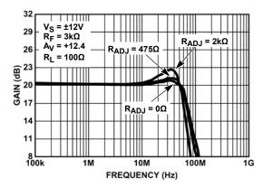
FIGURE 13. FREQUENCY RESPONSE FOR VARIOUS  $R_{\mbox{\scriptsize ADJ}}$
