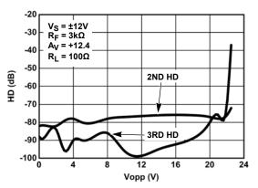
FIGURE 5. 200KHz 2ND AND 3RD HARMONIC DISTORTION vs VOLTAGE OUTPUT (FULL POWER MODE)
