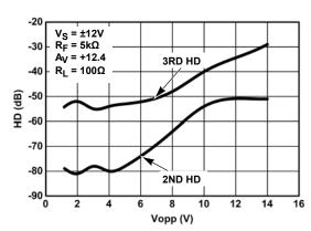
FIGURE 10. 3.75MHz 2ND AND 3RD HARMONIC DISTORTION vs OUTPUT VOLTAGE (HALF POWER MODE)
