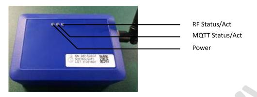
The Power light will be on anytime power is applied to the gateway. If this light is not lit, then there is no power to the gateway.
