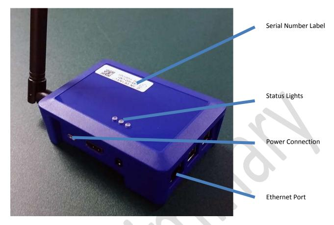
Every gateway is assigned a unique serial number at the factory. This serial number reflects the MAC address of the internal Whisker.IO Engine and is used to uniquely identify the gateway globally.
