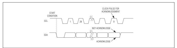
Figure 1. I<sup>2</sup>C Interface Timing Diagram
