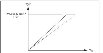
Figure 5. Limiter Gain Curve
