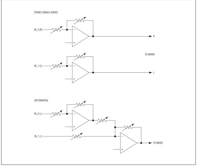
Figure 3. Differential and Stereo Single-Ended Input Configurations
