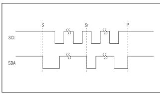
Figure 8. START, STOP, and REPEATED START Conditions
