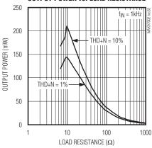
**Typical Operating Characteristics (continued)** (VLDOIN = VPVDD = 3.7V, VGND = VPGND = 0V. Single-ended inputs, preamp gain = 0dB, HPLVOL = HPRVOL = SPKVOL = 0dB. Speaker loads (ZSPK) connected between OUTP and OUTN. Headphone loads (RHP) connected from HPL or HPR to GND. ZSPK = ∞, RHP = ∞. CC1P-C1N = CHPVDD = CHPVSS = CBIAS = 1µF. TA = +25°C, unless otherwise noted.)
