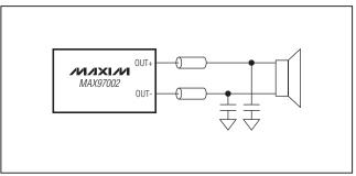
Figure 14. Optional Class D Ferrite Bead Filter
