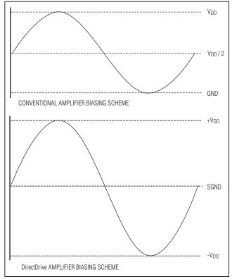
Figure 6.Traditional Amplifier Output vs. MAX97002 DirectDrive Output
