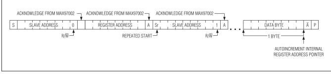
Figure 13. Reading n-Bytes of Data from the MAX97002
