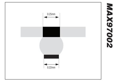
Figure 15. Recommended PCB Footprint
