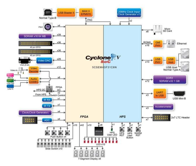
Figure 2-3 Block diagram of DE1-SoC
