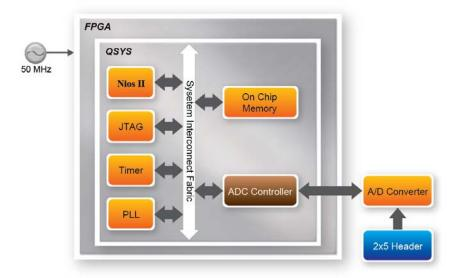
Figure 5-19 Block diagram of ADC reading
