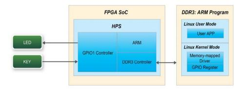
Figure 6-1 Block diagram of GPIO demonstration
