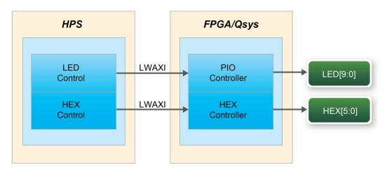
Figure 7-1 FPGA LED and HEX are controlled by HPS
