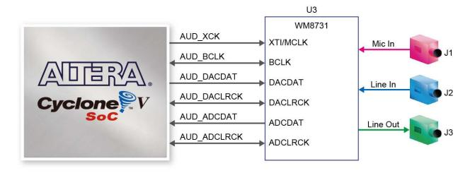
Figure 3-20 Connections between the FPGA and audio CODEC
