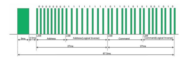
Figure 5-14 Typical frame of NEC protocol
