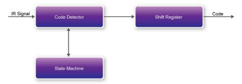
Figure 5-17 Modules in the IR Receiver controller
