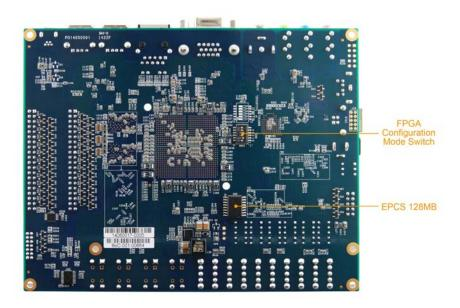
Figure 2-2 De1-SoC development board (bottom view)
