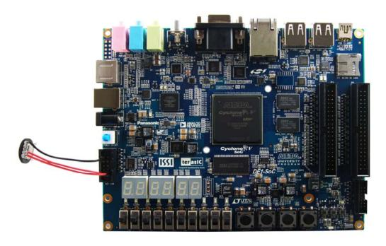
Figure 5-21 Hardware setup for the ADC reading demonstration
