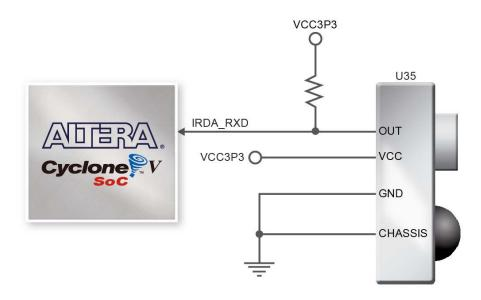
Figure 3-25 Connection between the FPGA and IR Receiver
