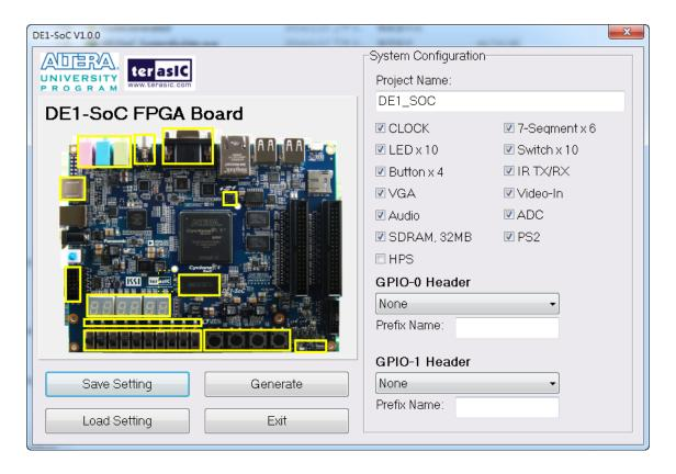
Figure 4-2 The GUI of DE1-SoC System Builder
