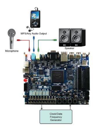
Figure 5-5 Setup for the Karaoke machine
