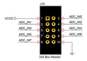
Figure 5-20 Pin distribution of the 2x5 Header for the ADC
