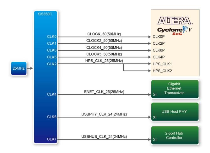
Figure 3-13 Block diagram of the clock distribution on DE1-SoC
