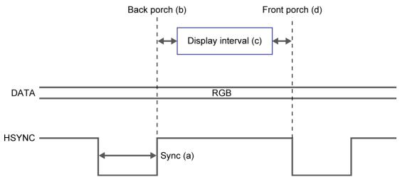
Figure 3-23 VGA horizontal timing specification
