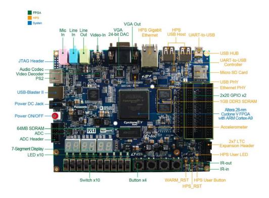
Figure 2-1 DE1-SoC development board (top view)
