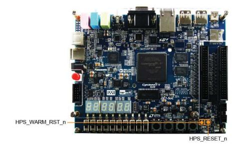
Figure 3-11 HPS cold reset and warm reset buttons on DE1-SoC
