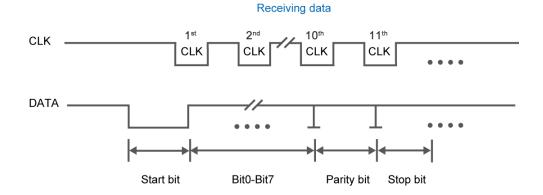
Figure 5-11 Waveform of clock and data signals during data transmission
