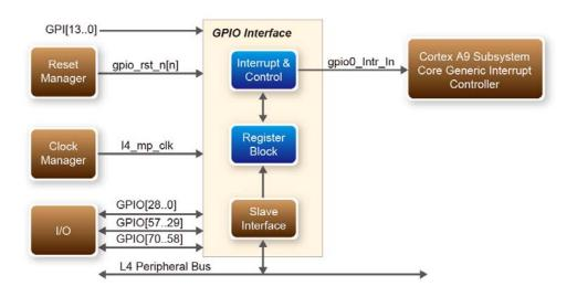
Figure 6-2 Block diagram of GPIO Interface
