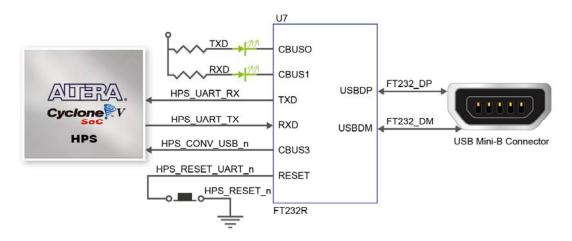
Figure 3-33 Connections between the HPS and FT232R Chip
