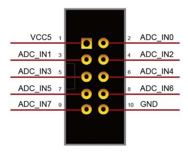
Figure 3-30 Signals of the 2x5 Header
