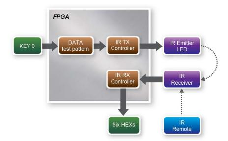
Figure 5-12 Block diagram of the IR emitter LED and receiver demonstration
