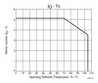
The motor current, I<sub>O</sub>, shown above represents the range of DC operation and chopping operation. The above graph shows performance when the overheating current control function (when pin 10 is connected to GND) is inoperational. For I<sub>O</sub> characteristics when overheating current control is operational, see I<sub>O</sub>-Tc characteristics given
