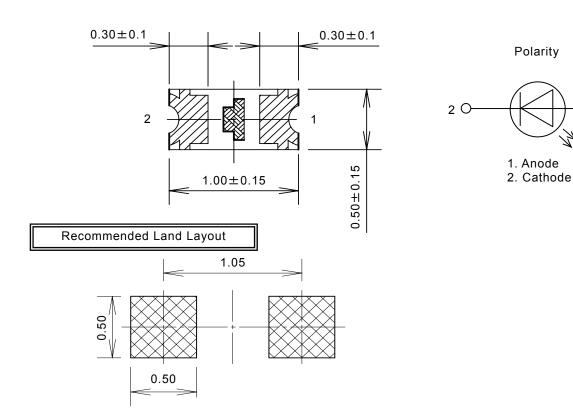
(Note1)Electrode projection is not included in the package dimensions.
