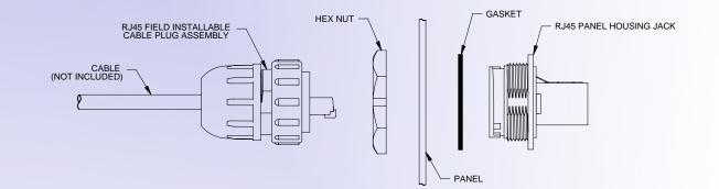
RJ45 FIELD INSTALLABLE CABLE PLUG ASSEMBLY (THREADED COUPLING)
