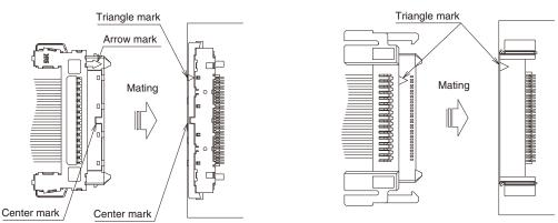
Additionally, this connector is equipped with reverse-insertion preventing mechanism, but a forced mating with a minimum force of 25N could damage the connector.
