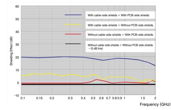
Notes :The measurement value of "Without plug-side shields + Without receptacle-side shields" are taken as the zero level of the graph vertical axis dB.
