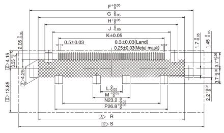
Note 1 : The coplanarity of the terminal leads is 0.1mm max. for all signal leads and 0.15mm max. for the shield leads.
