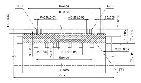
Note 1 : The coplanarity of the terminal leads is 0.1mm max.
