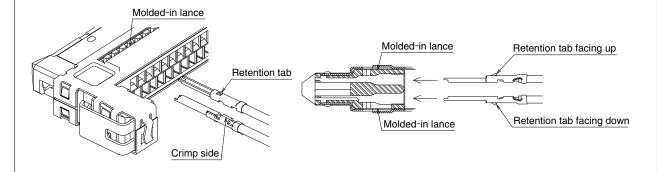
•Verify that the retention tabs clear the molded-in lances as shown on the illustration below.
