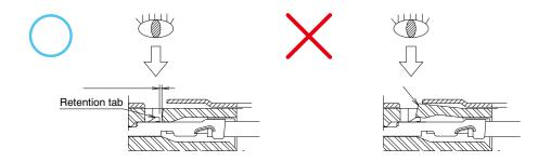
Light pull on the wire, with force NOT EXCEEDING 3N will also verify the correct contact insertion.
