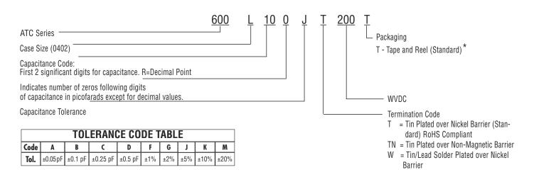
\*10,000 pieces on 7" reel, 4000 pieces on 7" reel and 500 pieces on prototype reel. Consult ATC for other options. The above part number refers to a 600L Series (case size L) 10 pF capacitor, J tolerance (±5%), 200 WVDC, with T termination (Tin Plated over Nickel Barrier, RoHS Compliant), Tape and Reel packaging.
