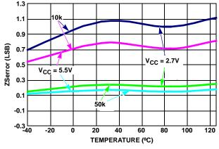
FIGURE 5. ZSerror vs TEMPERATURE
