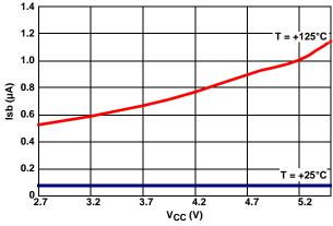
FIGURE 2. STANDBY ICC vs VCC
