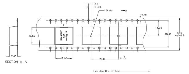
Supplied in tape and reel packaging, 350 parts per 13" diameter reel.
