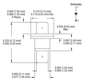
Dimensions are in inches (millimeters shown in parentheses)
