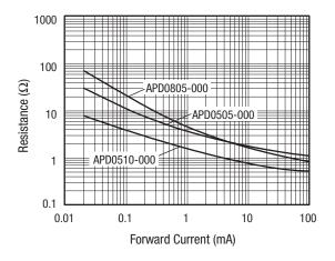
Figure 1. Resistance vs Forward Current @ 1 GHz
