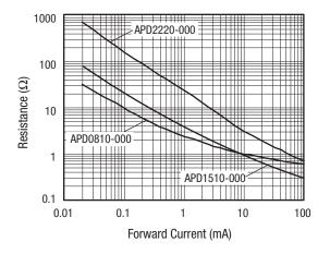
Figure 2. Resistance vs Forward Current @ 1 GHz
