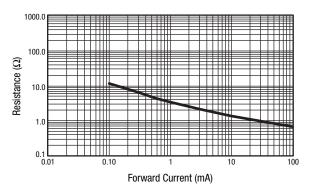
Figure 3. Resistance vs Forward Current @ 500 MHz (APD1505-000 Package)
