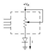
Two terminal Variable Resistor; Variable current
