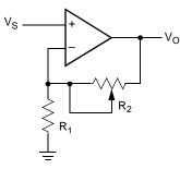
$V_0 = (1 + R_2/R_1)V_S$
