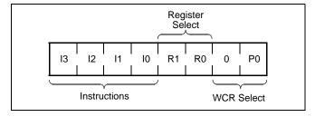
The four high order bits of the instruction byte specify the operation. The next two bits ( $R_1$  and  $R_0$ ) select one of the four registers that is to be acted upon when a register oriented instruction is issued. The last bit ( $P_0$ ) selects which one of the two potentiometers is to be affected by the instruction.
