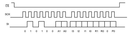
Figure 4. Three-Byte Command Sequence (Write)
