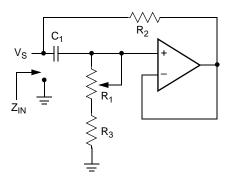
$\begin{aligned} Z_{\text{IN}} &= R_2 + s \; R_2 \; (R_1 + R_3) \; C_1 = R_2 + s \; \text{Leq} \\ & (R_1 + R_3) >> R_2 \end{aligned}$
