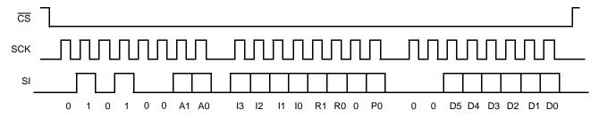
Figure 5. Three-Byte Command Sequence(Read)
