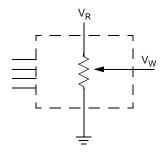
Three terminal Potentiometer; Variable voltage divider
