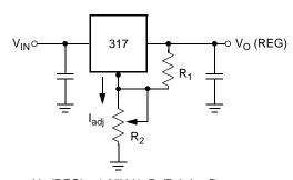
$V_O(REG) = 1.25V(1+R_2/R_1)+I_{adj}R_2$
