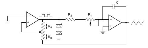
$\begin{array}{l} \text{frequency } \mu \ R_1, \ R_2, \ C \\ \text{amplitude } \mu \ R_A, \ R_B \end{array}$
