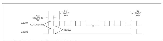
Figure 1. Free-Running Conversion Time and Rate Relationships
