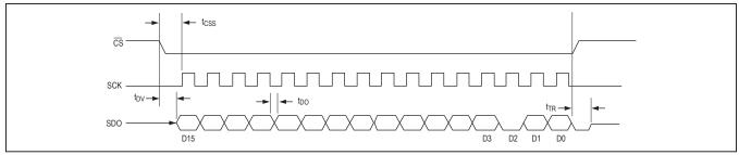
Figure 2. SPI Timing Diagram
