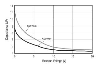
Figure 1. SMV2022 and SMV2023 Capacitance vs Reverse Voltage
