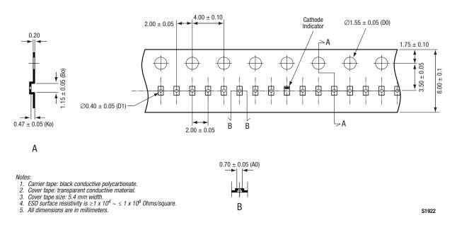
Figure 12. SOD-882 Tape and Reel Dimensions
