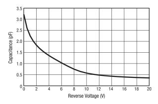
Figure 3. SMV2020-079LF Capacitance vs Reverse Voltage
