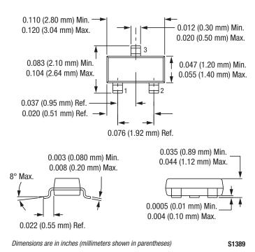
Figure 9. SOT-23 Package Dimensions
