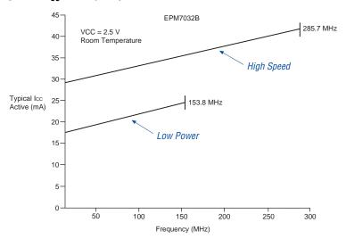
Figure 15. I<sub>CC</sub> vs. Frequency for EPM7032B Devices
