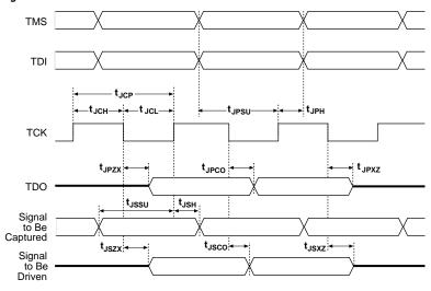
Figure 8. MAX 7000B JTAG Waveforms
