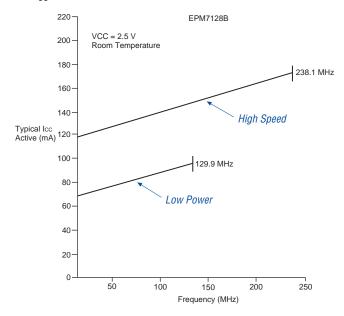
Figure 17.  $I_{CC}$  vs. Frequency for EPM7128B Devices
