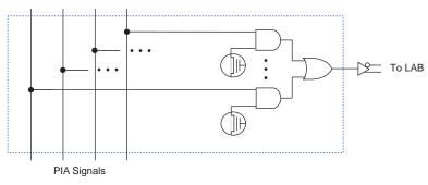
While the routing delays of channel-based routing schemes in masked or field-programmable gate arrays (FPGAs) are cumulative, variable, and path-dependent, the MAX 7000B PIA has a predictable delay. The PIA makes a design's timing performance easy to predict.
