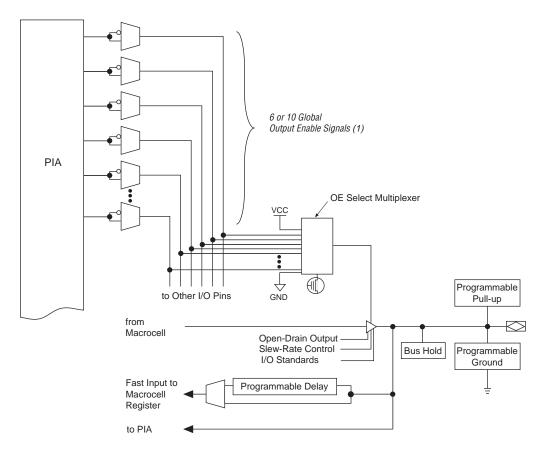
Figure 6. I/O Control Block of MAX 7000B Devices
