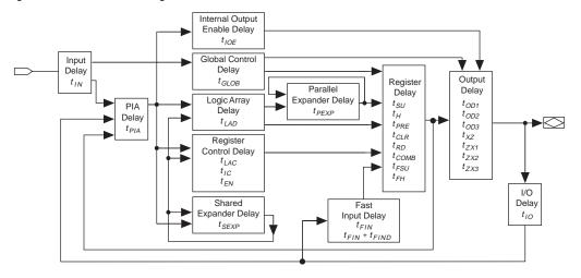
The timing characteristics of any signal path can be derived from the timing model and parameters of a particular device. External timing parameters, which represent pin-to-pin timing delays, can be calculated as the sum of internal parameters. Figure 14 shows the timing relationship between internal and external delay parameters.
