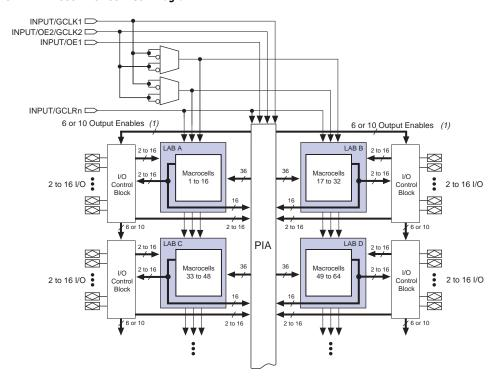
Figure 1. MAX 7000B Device Block Diagram
