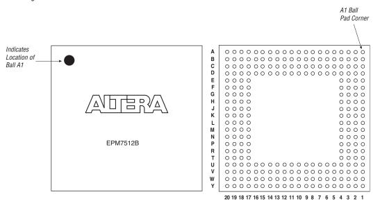
Figure 29. 256-Pin FineLine BGA Package Pin-Out Diagram
