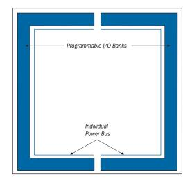
Figure 9. MAX 7000B I/O Banks for Various Advanced I/O Standards
