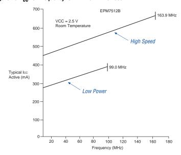
Figure 19.  $I_{CC}$  vs. Frequency for EPM7512B Devices
