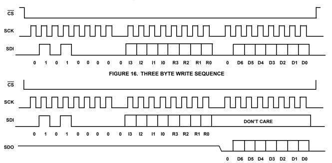
FIGURE 17. THREE BYTE READ SEQUENCE
