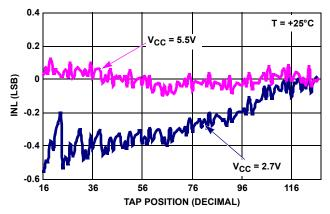
FIGURE 8. INL vs TAP POSITION IN RHEOSTAT MODE FOR  $10 \mathrm{k}\Omega$  (W)
