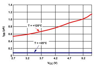
FIGURE 2. STANDBY I<sub>CC</sub> vs V<sub>CC</sub>
