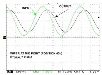
FIGURE 12. FREQUENCY RESPONSE (2.6MHz)
