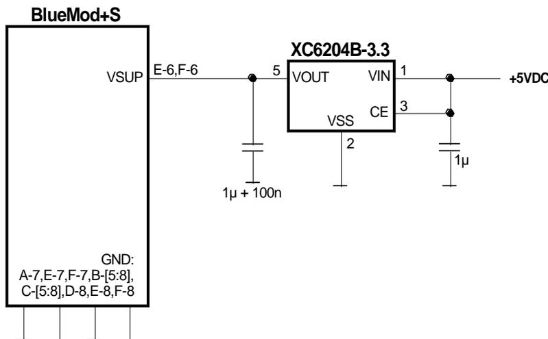
Figure 2: BlueMod+S Example Power Supply with LDO
