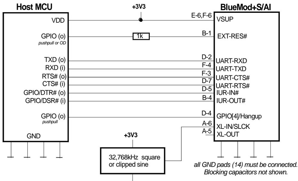
*The oscillator is optional. Leave A-6 open if the oscillator is not present. You can also connect an 32,768kHz XTAL and two capacitors at A-6 and A-5.*
