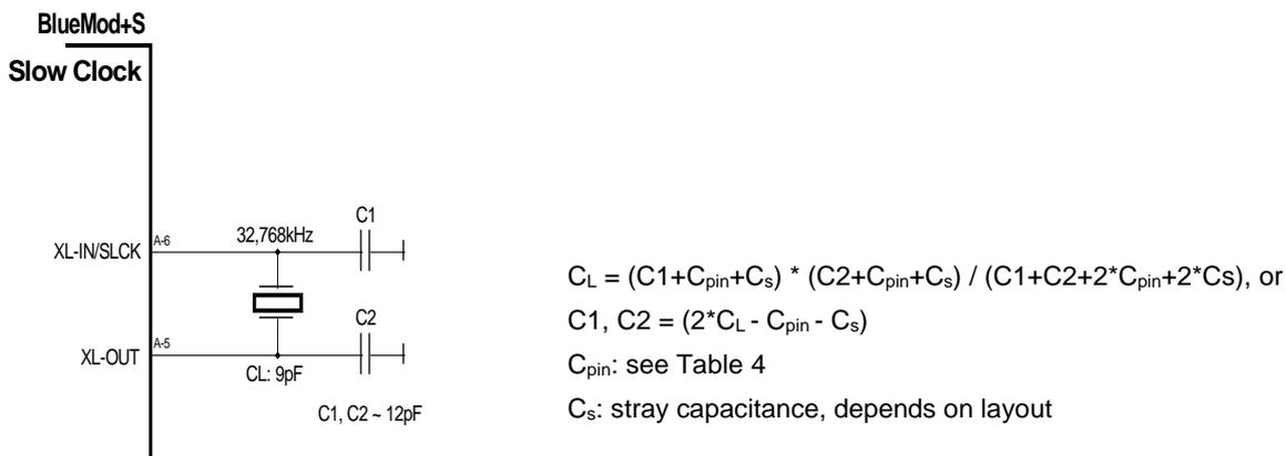
Figure 10: BlueMod+S connection of external XTAL
