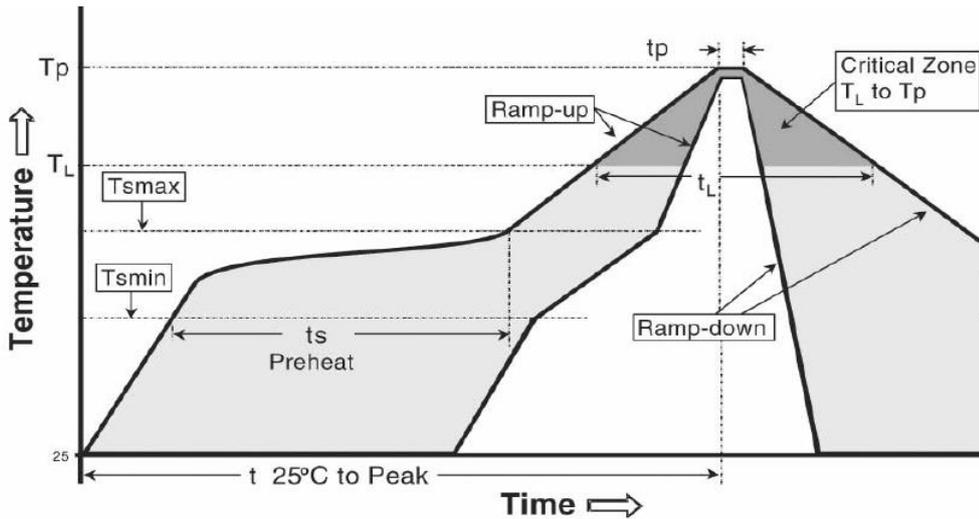
Figure 18: Soldering Temperature-Time Profile (For Reflow Soldering)
