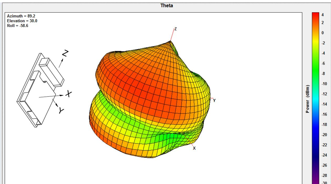
Figure 13: Typical Antenna Radiation Pattern at 2402MHz
