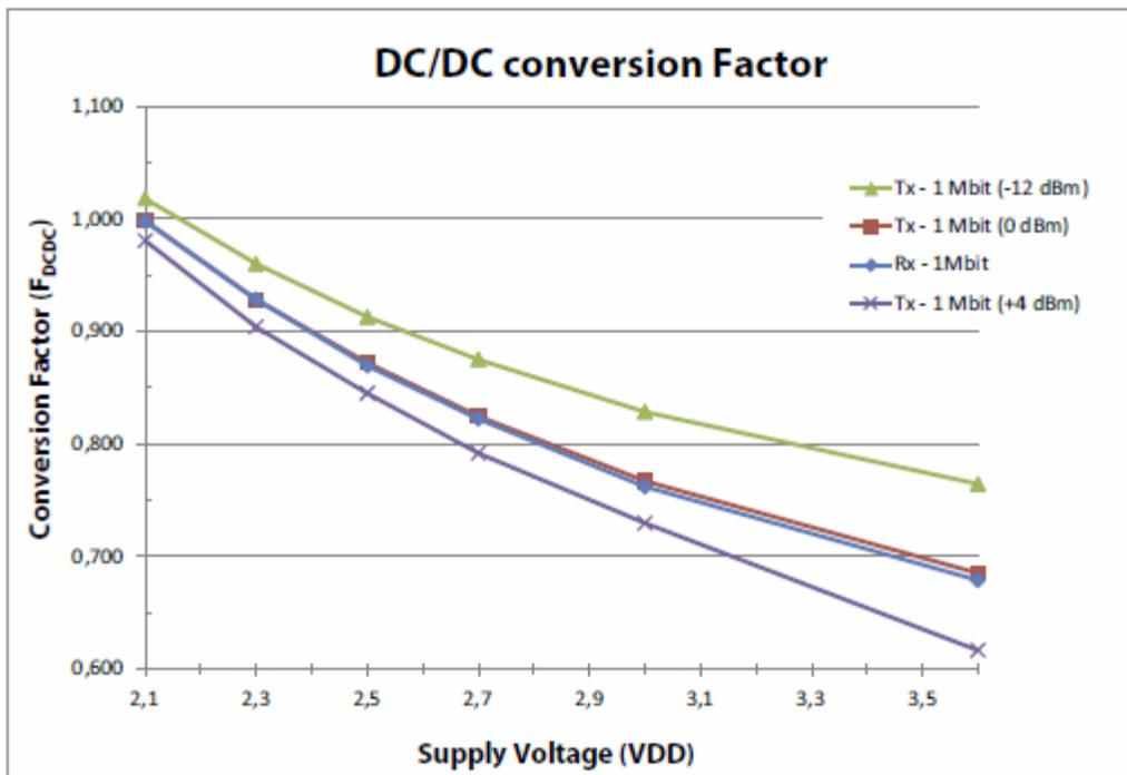
Figure 11: DC/DC Conversion Factor  $F_{DCDC}$  versus Supply Voltage
