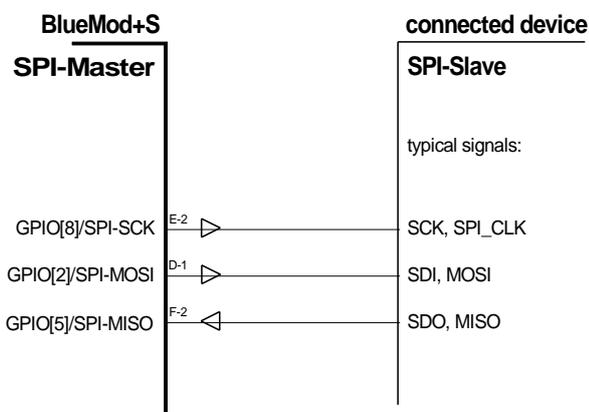
Figure 9: BlueMod+S SPI Interface (Example: Master Mode)
