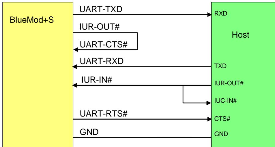
Figure 5: Five Wire Interface supporting UICP (Minimum Signals needed)
