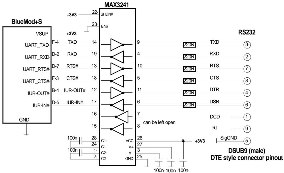
Figure 6: BlueMod+S Example Serial Interface (RS-232) Supporting UICP
