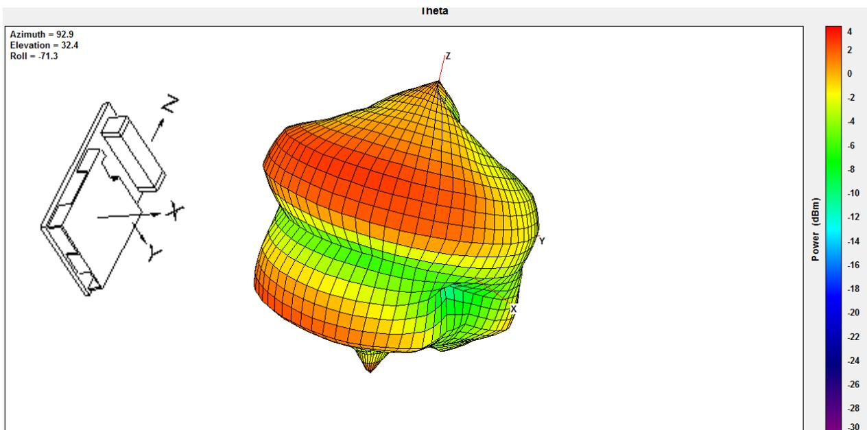
Figure 15: Typical Antenna Radiation Pattern at 2480MHz
