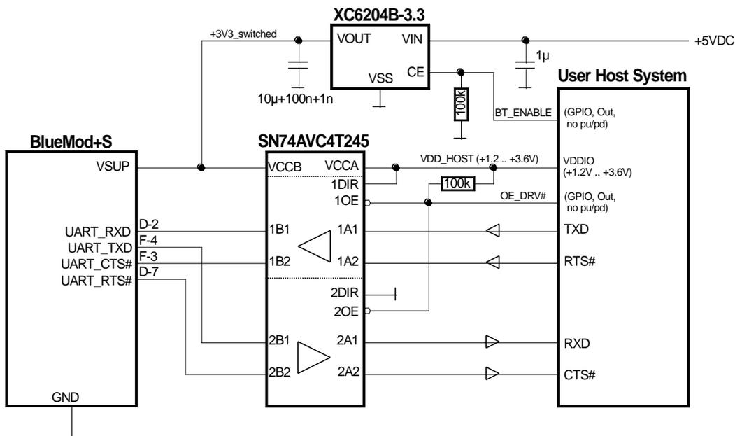
Figure 7: BlueMod+S Example Serial Interface (Mixed Signal Level)
