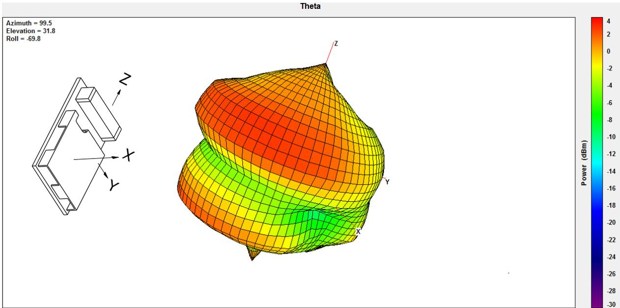
Figure 14: Typical Antenna Radiation Pattern at 2441MHz
