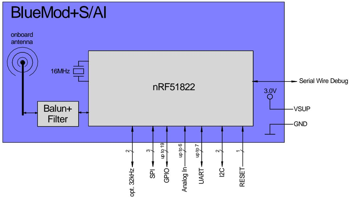
Figure 1: BlueMod+S/AI Block Diagram
