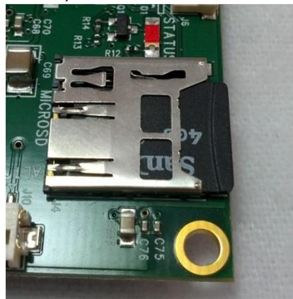
To remove the microSD card, press the card back into the socket until another “click” sound is heard, then release pressure on the card. At this point, the card should be partially ejected from the socket. Finally grab the card and gently pull to remove it. See the following pictures for proper micro-SD removal:
