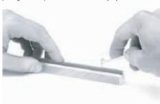
3. With firm steady pressure, push the contact into the cavity until the resilient internal shoulder snaps into the locking groove in the contact. To prevent over insertion, the tool tip bottoms against the rear of the insulator.
