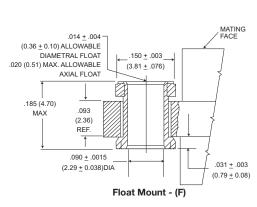
Shown here is a cutaway view of the float mount for the MD connector. The basic shell dimensions are the same for the float mount and the screw mounting hole configurations. View shown is for standard float mount front panel mounting. Reverse mounting is available on request.
