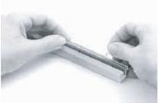
1. Place the connector into the slot in the assembly block with the arrows on the insulator pointing downward. The connector will bottom against the internal shoulder in the groove in the assembly block. Start contact insertion by placing the crimped contact in the cavity by hard.
