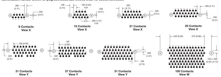
All Termination Configurations .100 (2.54)  $\times$  .100 (2.54) Grid Pattern, Offset .050 (1.27).
