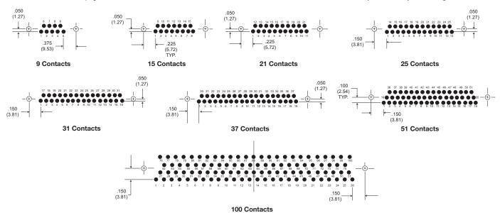
NOTE: Standard lead termination is #24 AWG, solid copper, solder or tin dipped All Termination Configurations .100 (2.54) x .100 (2.54) Grid Pattern, Offset .050 (1.27)
