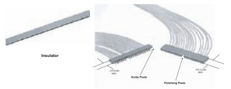
The guide posts and polarizing posts are inserted in the same manner as the contacts. The guide posts are inserted into the socket insulator and the polarizing posts are inserted into the pin insulator. The corresponding contact in the mating insulator must be removed for each. See assembly instructions.
