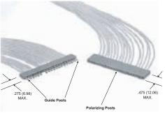
4. The guide post and polarizing posts are inserted in teh same manner as the contacts. The guide posts are inserted into the socket insulator, and the polarizing posts are inserted into the pin insulartor. The corresponding contact in the mating insulator must be removed for each.
