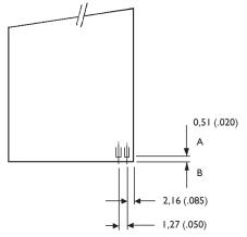
Diagram 2 illustrates how the connector is prepared with short pigtails and a special first pot which just captures the contacts. The final back potting for strength is controlled by our standard 7,00 (.275) potting fixtures.
