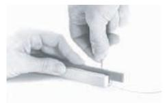
2. Position the insertion tool tip on the rear of contact as shown. The insulation must be pulled back from the crimp pot approximately 1/32" to allow the tool tip to butt against the contact crimp pot.
