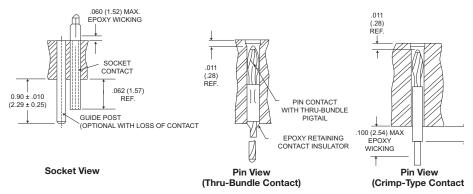
NOTE: Guide posts can be installed in any contaact cavity for polarization purposes.
