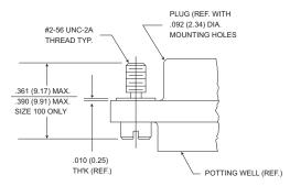
Figure 1. Jackscrew - Low profile Slotted Head Size 9-51
