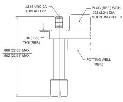
Figure 2. Jackscrew - High Profile Slotted Head Size 9-51 Size 100\*
