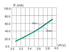
FIG.1 FORWARD CURRENT VS. FORWARD VOLTAGE.
