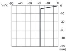
FIG.3 REVERSE CURRENT VS. REVERSE VOLTAGE.
