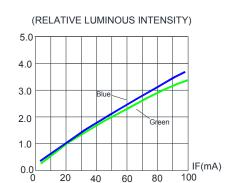
FIG.2 RELATIVE LUMINOUS INTENSITY VS. FORWARD CURRENT
