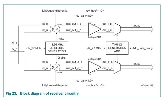
The receiver can also be operated in a single ended mode. In this case the Rcv\_RX\_single bit has to be set. In the single ended mode, the two receiver pins RXP and RXN need to be connected together and will provide a single ended signal to the receiver circuitry.
