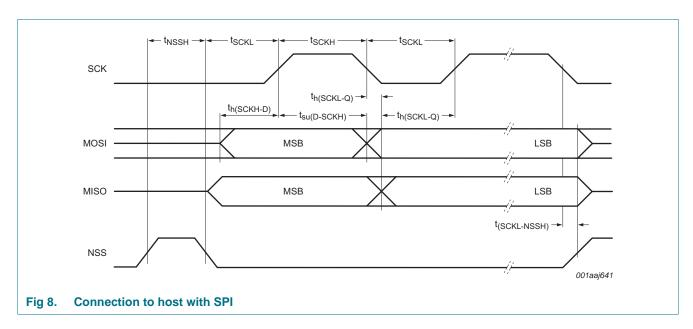
**Remark:** To send more bytes in one data stream the NSS signal must be LOW during the send process. To send more than one data stream the NSS signal must be HIGH between each data stream.
