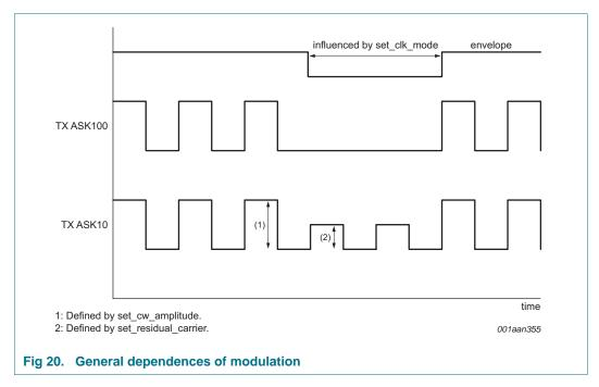
Note: When changing the continuous carrier ampliture, the residual carrier amplidude also changes, while the modulation index remains the same.
