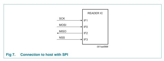
The MFRC630 acts as a slave during the SPI communication. The SPI clock SCK has to be generated by the master. Data communication from the master to the slave uses the Line MOSI. Line MISO is used to send data back from the MFRC630 to the master.
