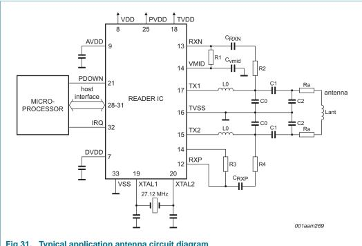
Fig 31. Typical application antenna circuit diagram
