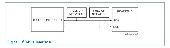
SDA is a bidirectional line, connected to a positive supply voltage via a pull-up resistor. Both lines SDA and SCL are set to HIGH level if no data is transmitted. Data on the  $I^2C$ -bus can be transferred at data rates of up to 400 kbit/s in fast mode, up to 1 Mbit/s in the fast mode+.
