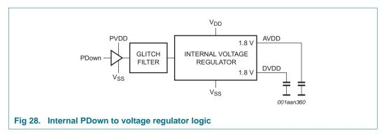
This internal procedure consists of two phases:
