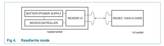
A typical system using the MFRC630 is using a microcontroller to implement the higher levels of the contactless communication protocol and a power supply (battery or external supply).
